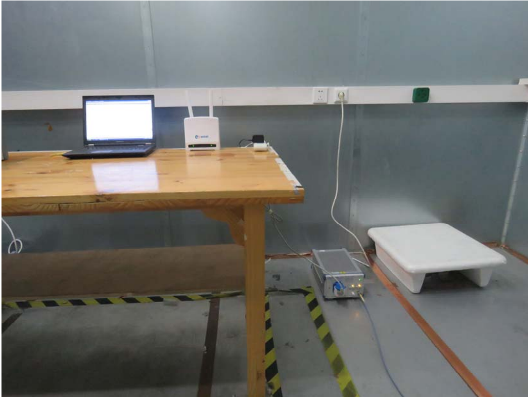
Picture 3 Conducted Emission Test Setup
