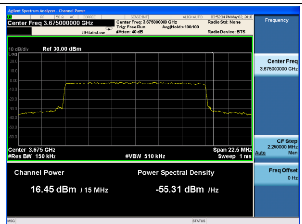
LTE Band 43 16QAM 15MHz CH44340
