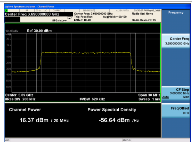
LTE Band 43 16QAM 20MHz CH44490
