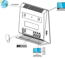
Step 1 Connect the power adapter to the CPE.
