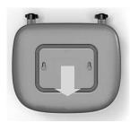
2. Insert the battery by aligning the metal contacts on the battery with the metal contacts in the battery compartment. Gently push down on the battery until it clicks into place.
