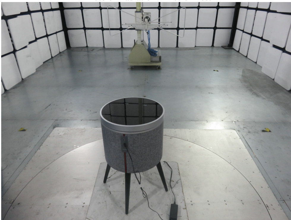
Photo of Radiation Emission Test
