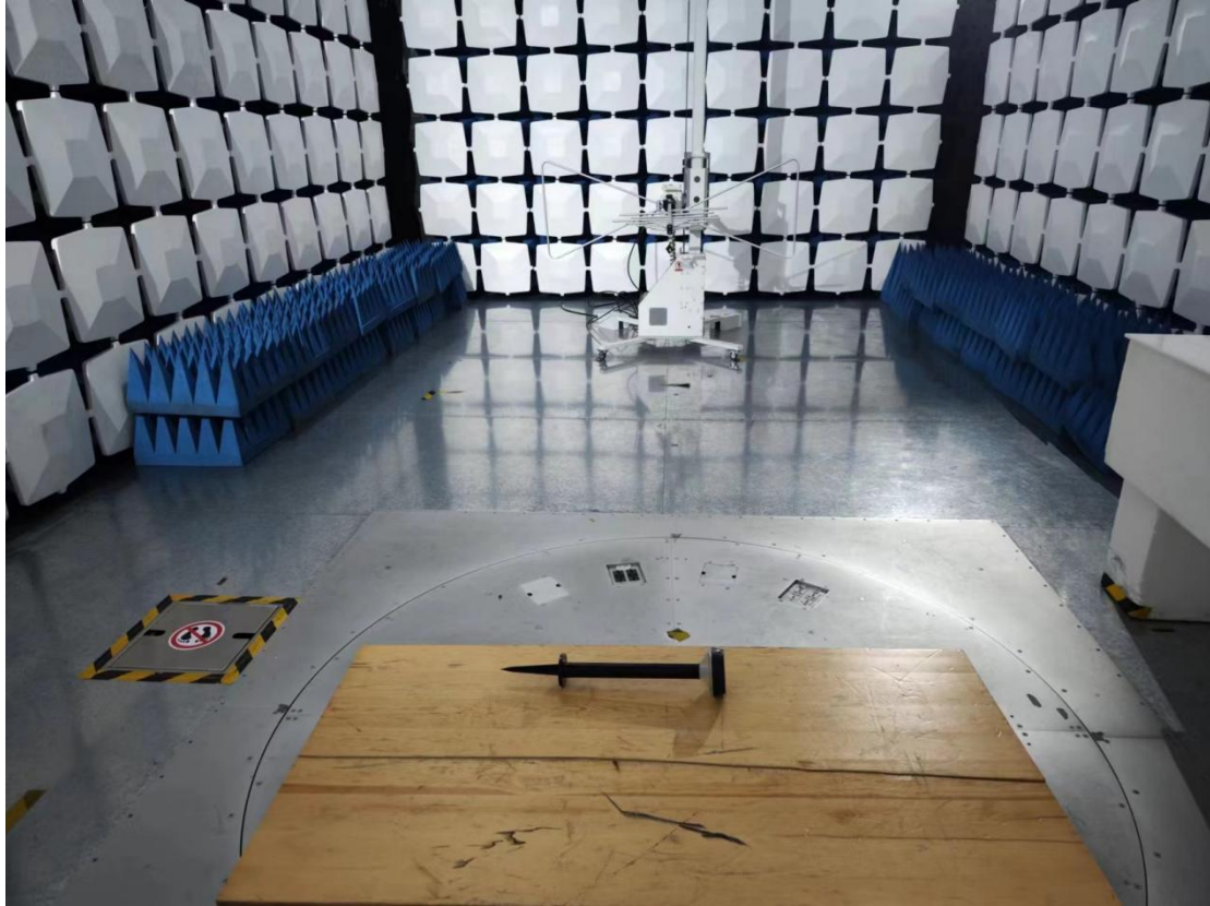
Blow 1GHz for radiated emission test setup
