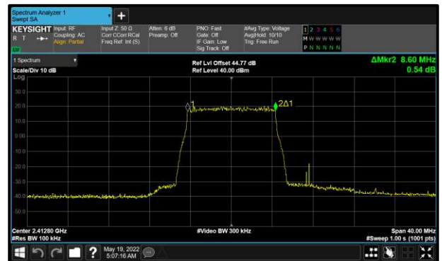
Figure 20 - LTE Full Resource Blocks 9 MHz BW Maximum 99% OBW
