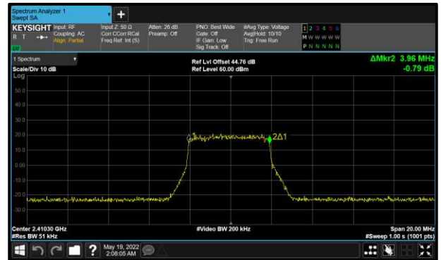
Figure 18 - LTE Full Resource Blocks 4.5 MHz BW Maximum 99% OBW
