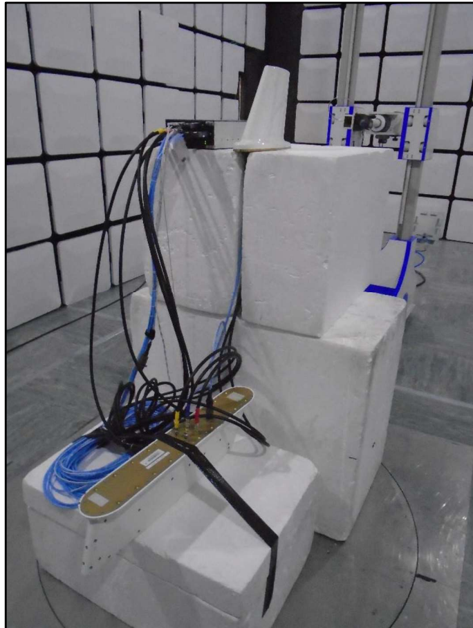
Figure 100 - Test Setup - 18 GHz to 25 GHz
