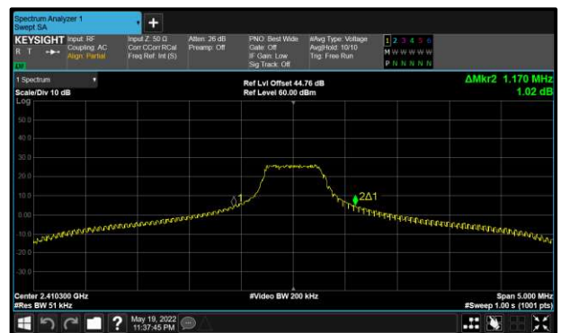
Figure 12 - LTE 3 Resource Blocks B 4.50 MHz Maximum 99% OBW
