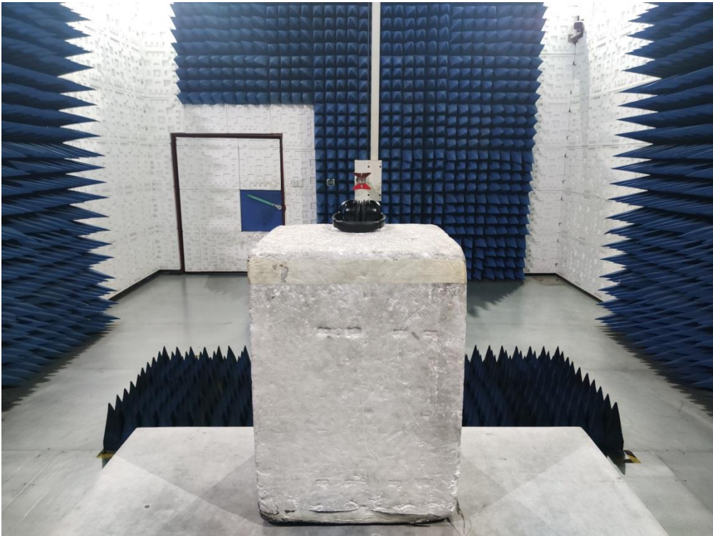
RADIATED EMISSION TEST SETUP ABOVE 1GHz
