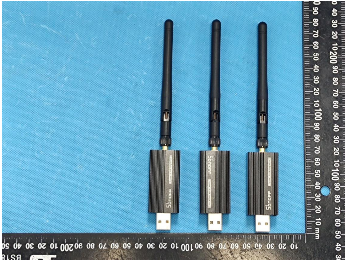
With Serial Chip: CP2102N-QFN28
