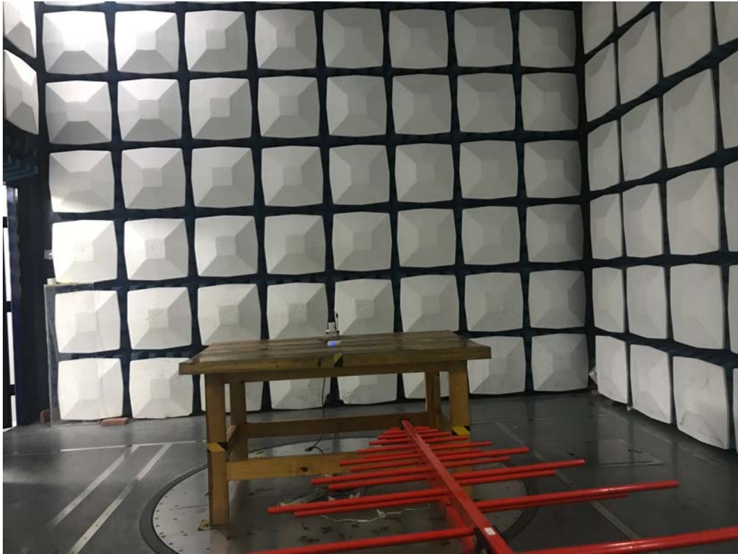
Radiated Emission Above 1GHz View
