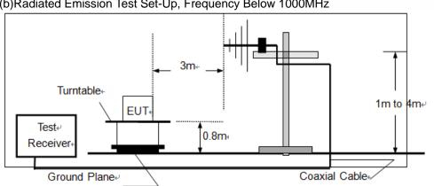
(b)Radiated Emission Test Set-Up, Frequency Below 1000MHz
