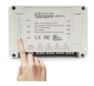
2. Press and hold one of the 4 ON/OFF buttons for 7 seconds until the wifi LED fast blinks 3 times and repeat.
