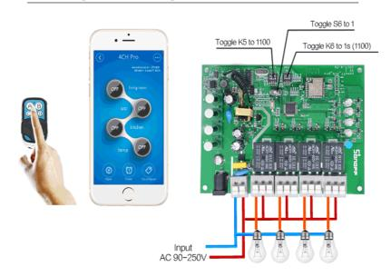
2. In inching mode, you can turn on the connected devices for 0.25-4s. For example, you can turn on CH1 connected device for 1s, then auto-off.
