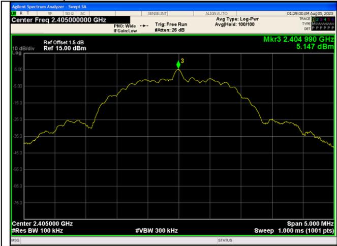
In-Band Reference Level Zigbee 2405
