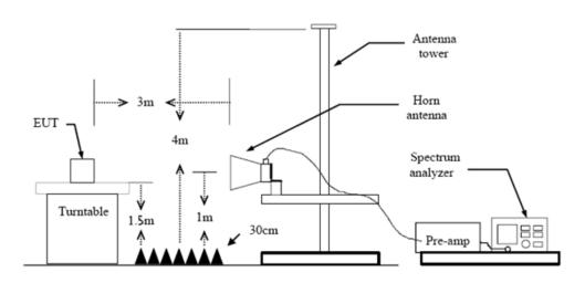
Above 1GHz Test Setup
