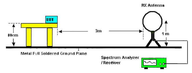
Below 30MHz Test Setup
