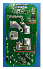
S40ZBTPB is different from S40ZBTPB Lite in that there is an electric quantity measurement and detection circuit, the rest are the same.
