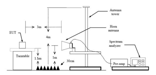
Above 1GHz Test Setup
