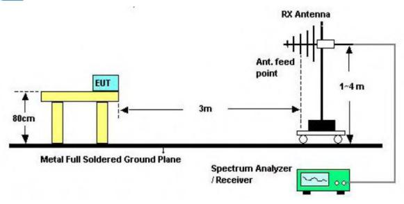
30-1000MHz Test Setup
