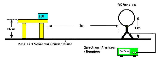
Below 30MHz Test Setup
