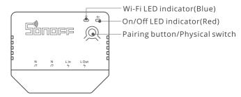
① The device weight is less than 1 kg. The installation height of less than 2 m is recommended.
