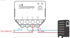
The wiring instruction of single L wire (connect to the S-MATE switch):
