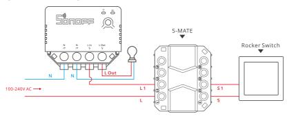
One S-MATE can be connected to one 3-gang switch at most. The control way to connecting each gang and MINIR3 can be one-to-more, more-to-one and more-to-more. There are L/L1/L2/L3 on the S-MATE which can be used as terminal connectors, but you have options to directly connect the L wire of MINIR3 to the L wire in the switching box without going through the S-MATE.
