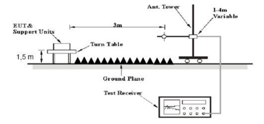
The radiated emissions were performed in the 3 meters distance, using the setup accordance with the ANSI C63.10-2013. The specification used was the FCC 15.209, and FCC 15.249 limits.
