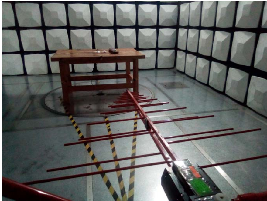
Radiated Emission View (Below 1GHz)
