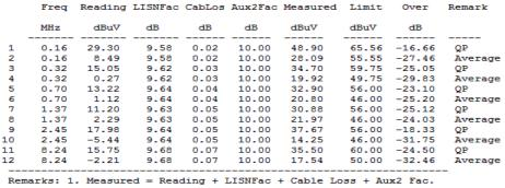
emarks: 1. Measured = Reading + LISNFac + Cable Loss + Aux2 Fac.
