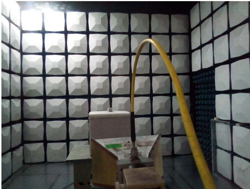
Radiated Emission View (Above 1GHz)
