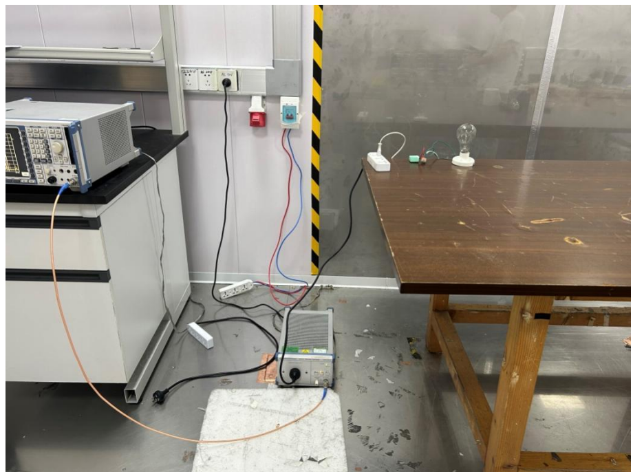
Conducted Emission Test Setup
