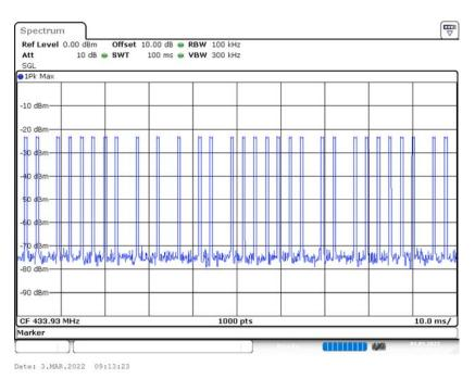
The graph shows the duration of 'on' signal. From Marker 1 to Delta 2, duration is 100ms.
