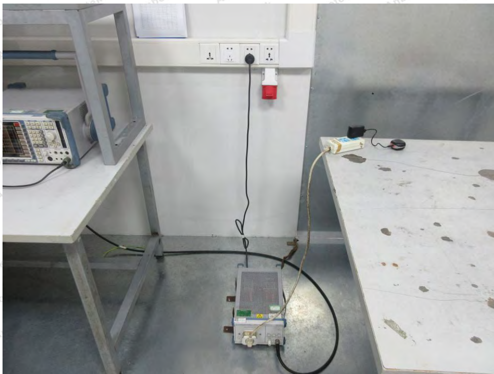
Photo of Conducted Emission Measurement
