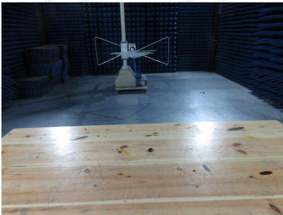
Photo of Radiation Emission Test
