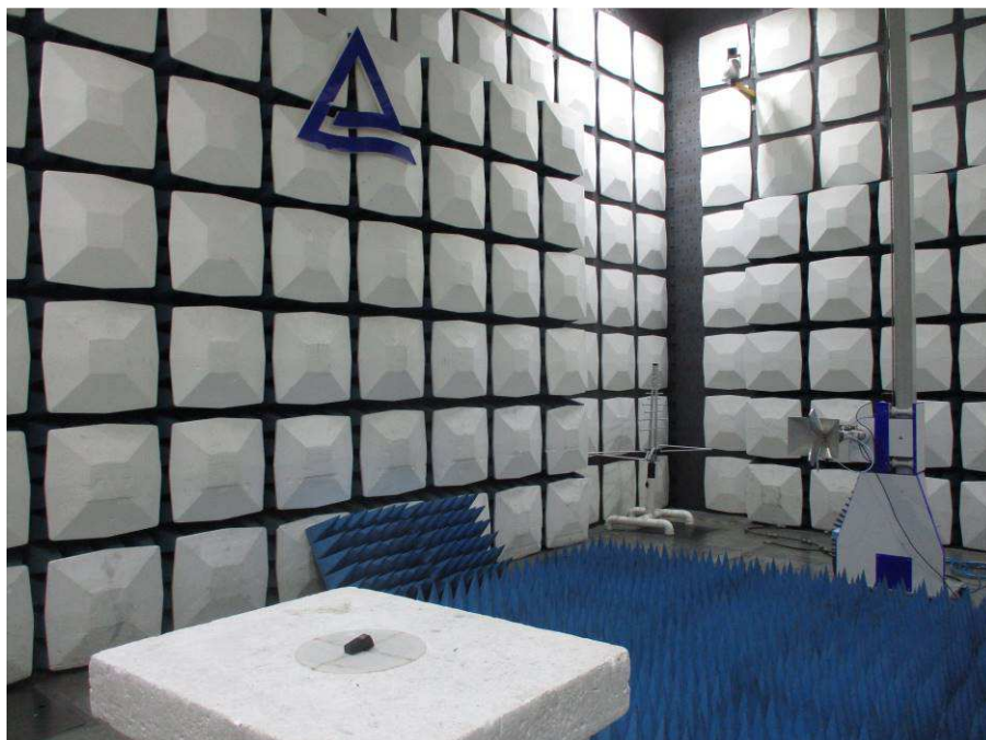
Photograph 4: Set-up photo for Radiated Emissions Above 1GHz
