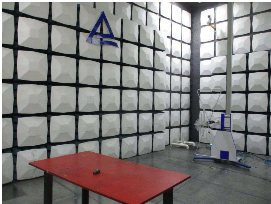
Photograph 3: Set-up photo for Radiated Emissions Below 1GHz
