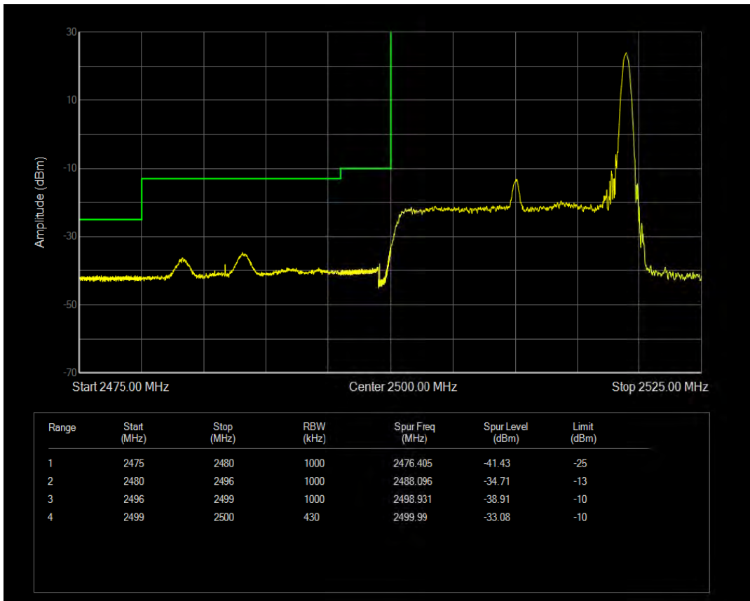
LTE Band7 QAM16 BW=20MHz Channel=20850 RB Size=1 Position=#0
