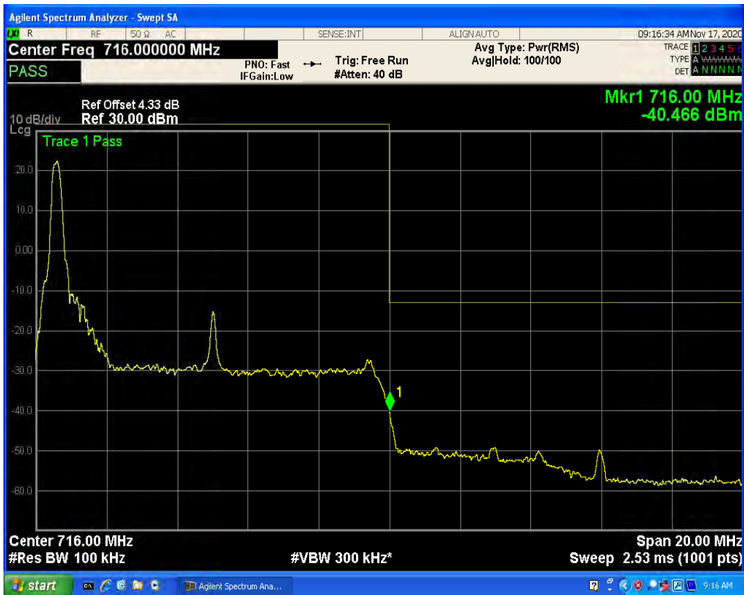
LTE Band17 QPSK BW=10MHz Channel=23800 RB Size=1 Position=#Max
