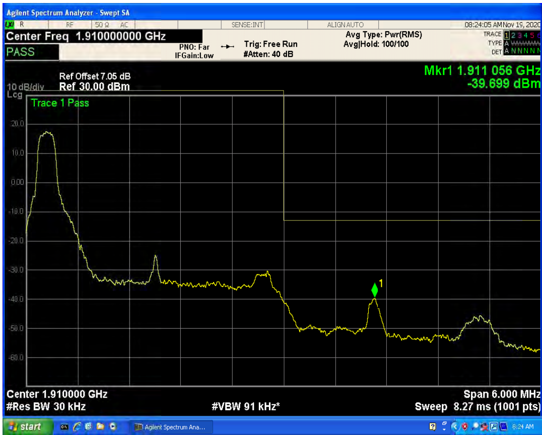
LTE Band2 QPSK BW=3MHz Channel=19185 RB Size=1 Position=#Max
