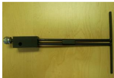
Figure 1 – MVG COMOSAR Validation Dipole
