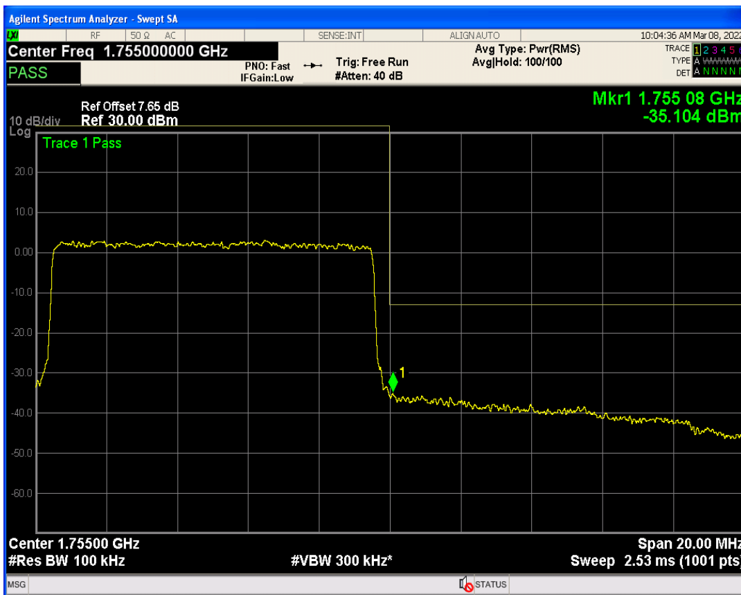
Band4 QPSK BW=15MHz Channel=20025 RB Size=1 Position=#0
