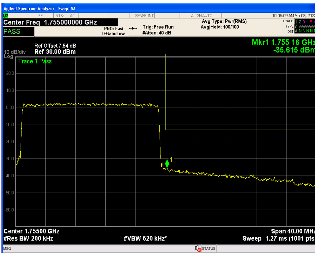
Band5 QPSK BW=1.4MHz Channel=20407 RB Size=1 Position=#Max
