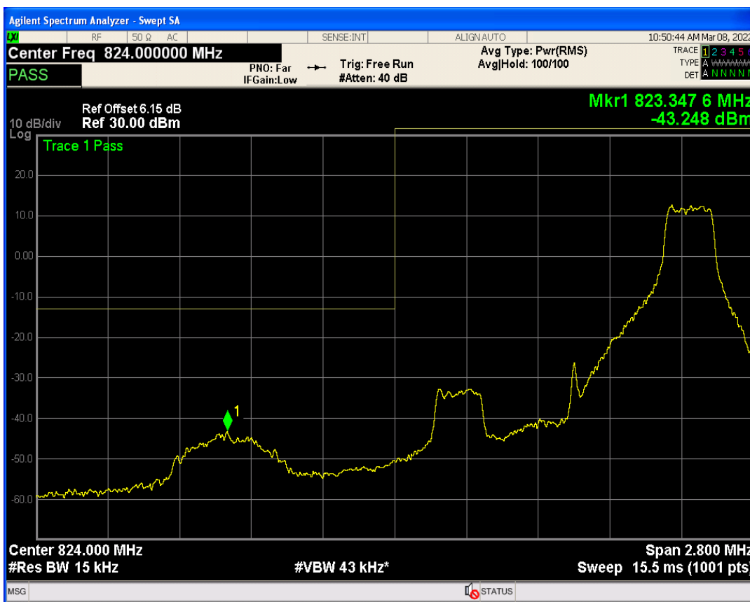
Band5 QPSK BW=1.4MHz Channel=20643 RB Size=1 Position=#0
