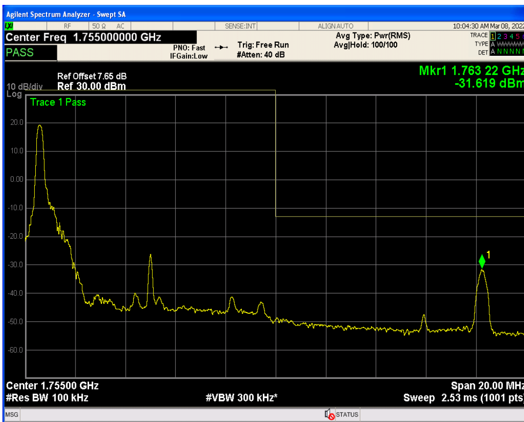
Band4 QAM16 BW=10MHz Channel=20350 RB Size=1 Position=#Max
