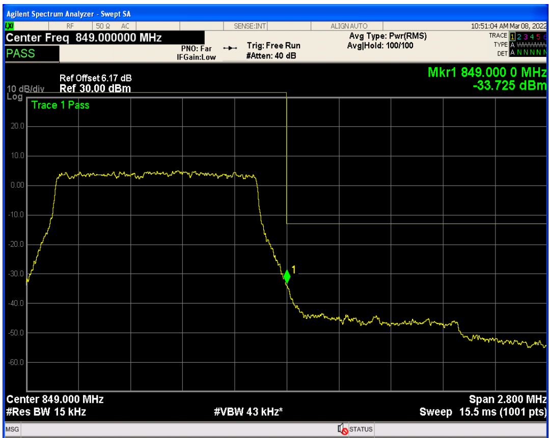
Band5 QAM16 BW=1.4MHz Channel=20643 RB Size=1 Position=#Max
