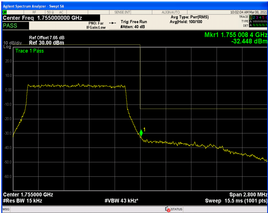
Band4 QAM16 BW=1.4MHz Channel=20393 RB Size=1 Position=#Max
