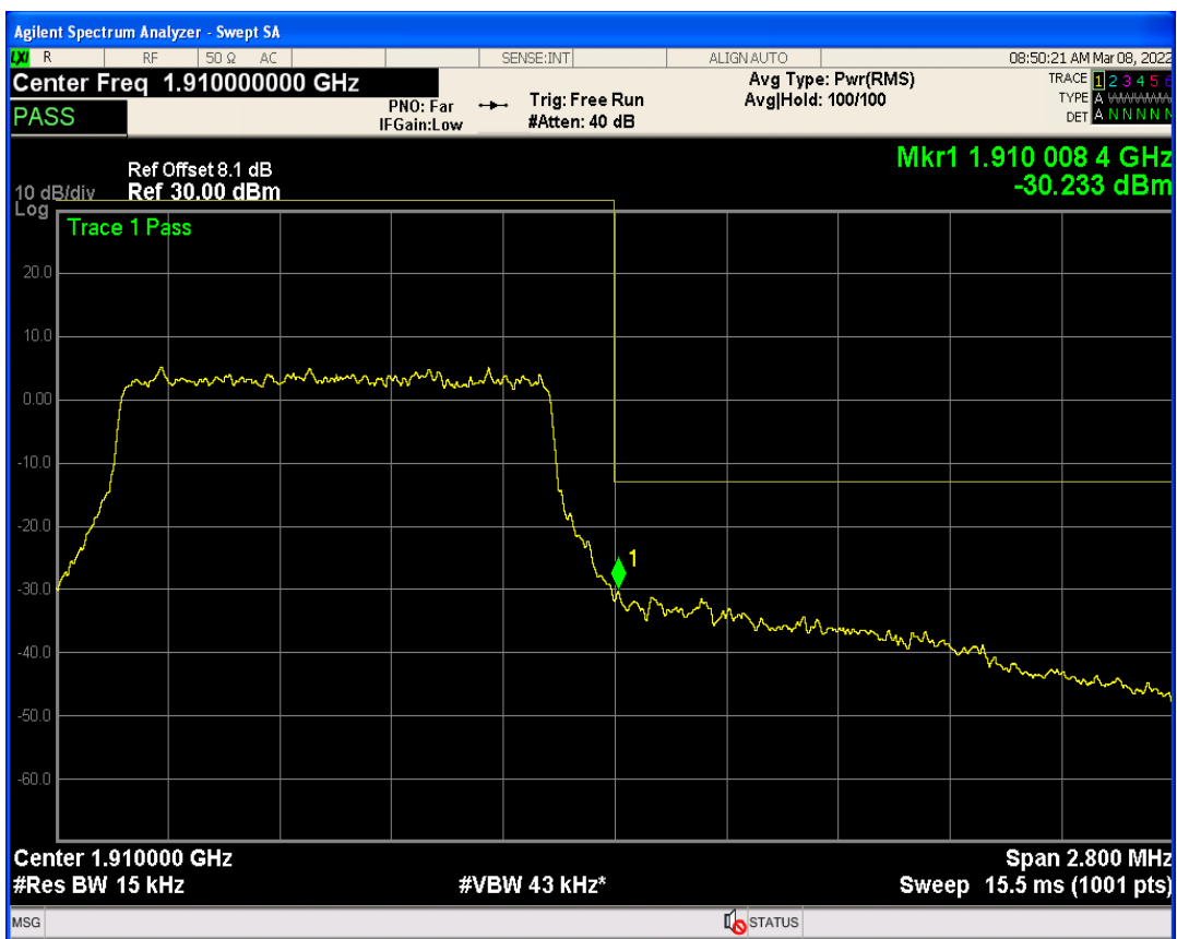
Band2 QPSK BW=3MHz Channel=18615 RB Size=1 Position=#Max
