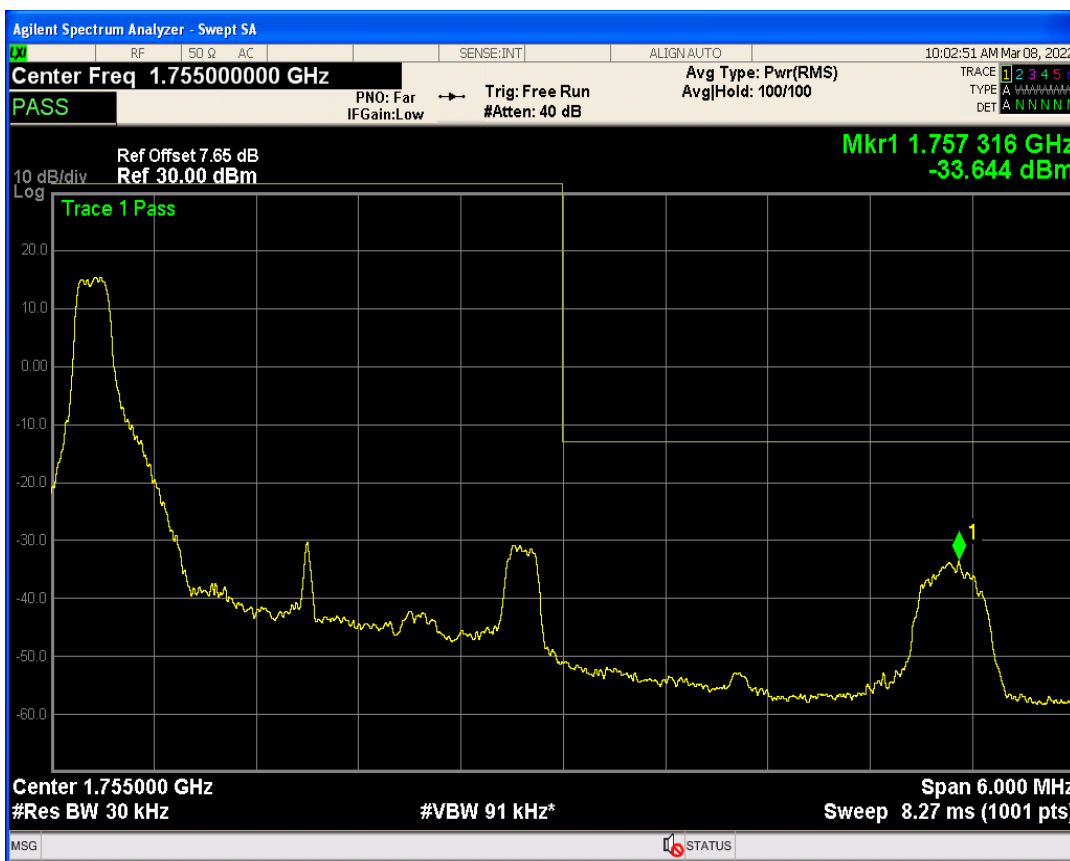
Band4 QAM16 BW=3MHz Channel=20385 RB Size=1 Position=#Max
