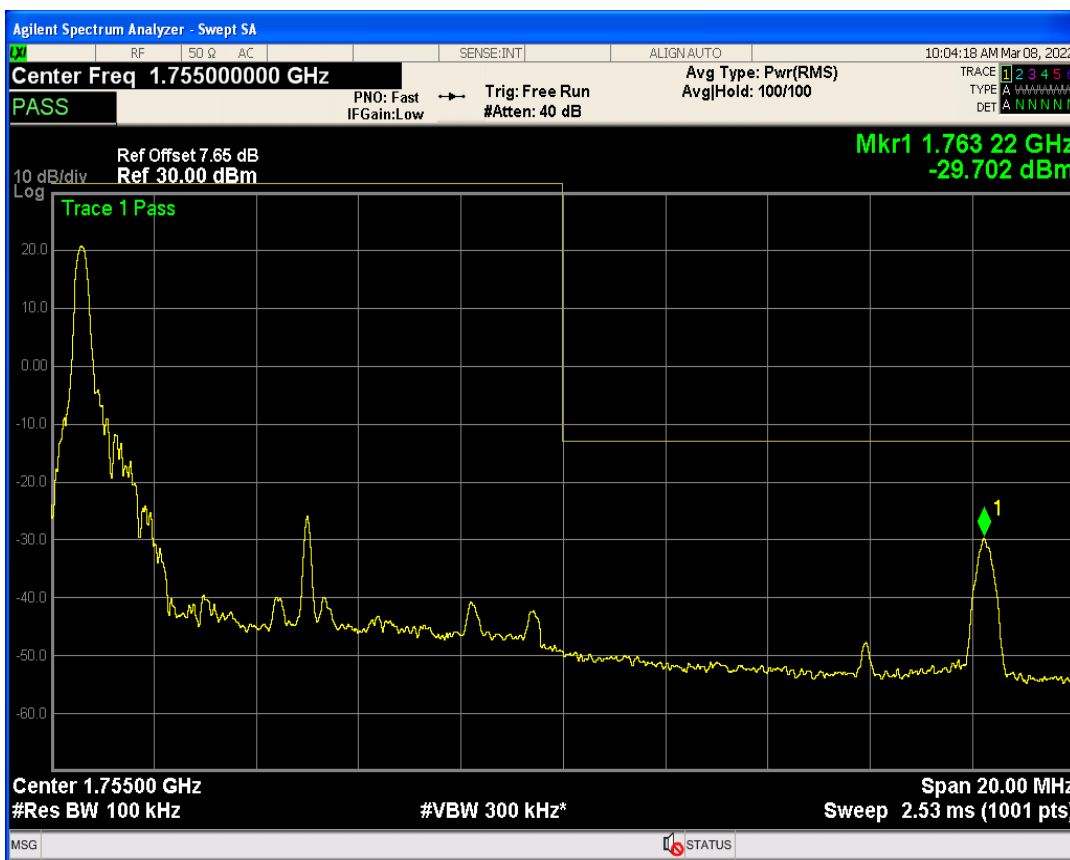
Band4 QPSK BW=10MHz Channel=20350 RB Size=50 Position=#0
