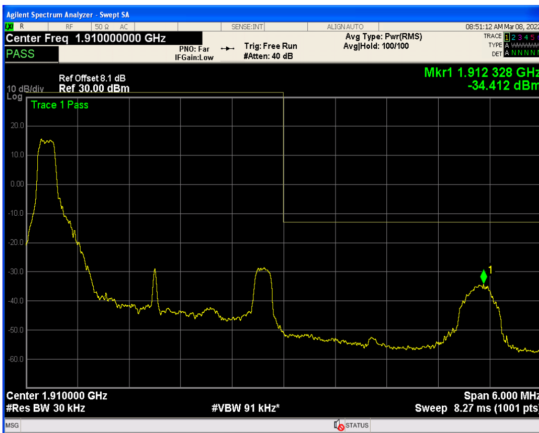
Band2 QAM16 BW=3MHz Channel=19185 RB Size=1 Position=#Max
