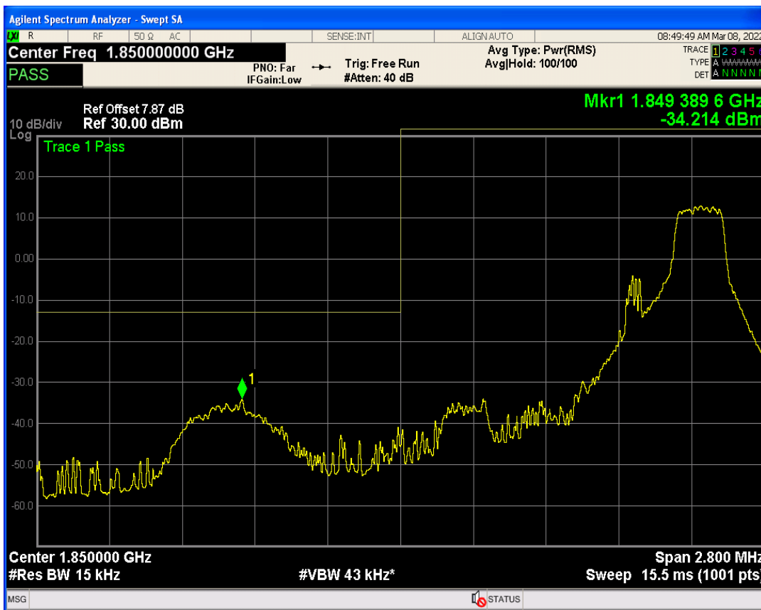
Band2 QPSK BW=1.4MHz Channel=19193 RB Size=1 Position=#0
