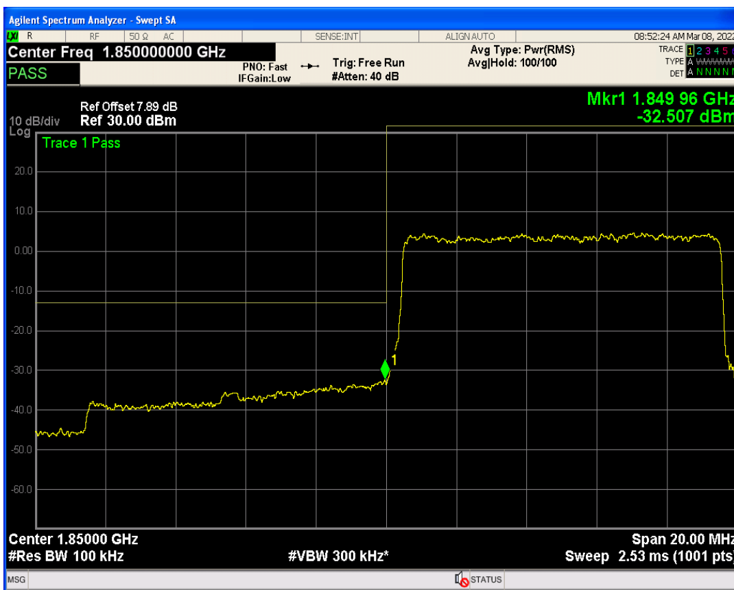
Band2 QPSK BW=10MHz Channel=18650 RB Size=1 Position=#Max
