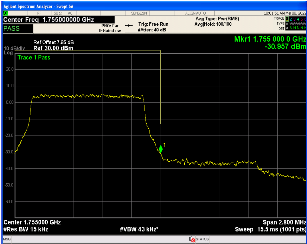
Band4 QAM16 BW=1.4MHz Channel=20393 RB Size=6 Position=#0
