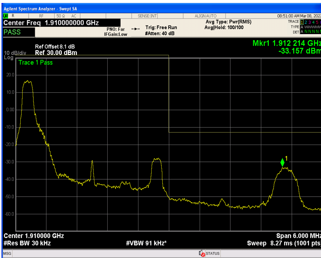
Band2 QPSK BW=3MHz Channel=19185 RB Size=1 Position=#Max
