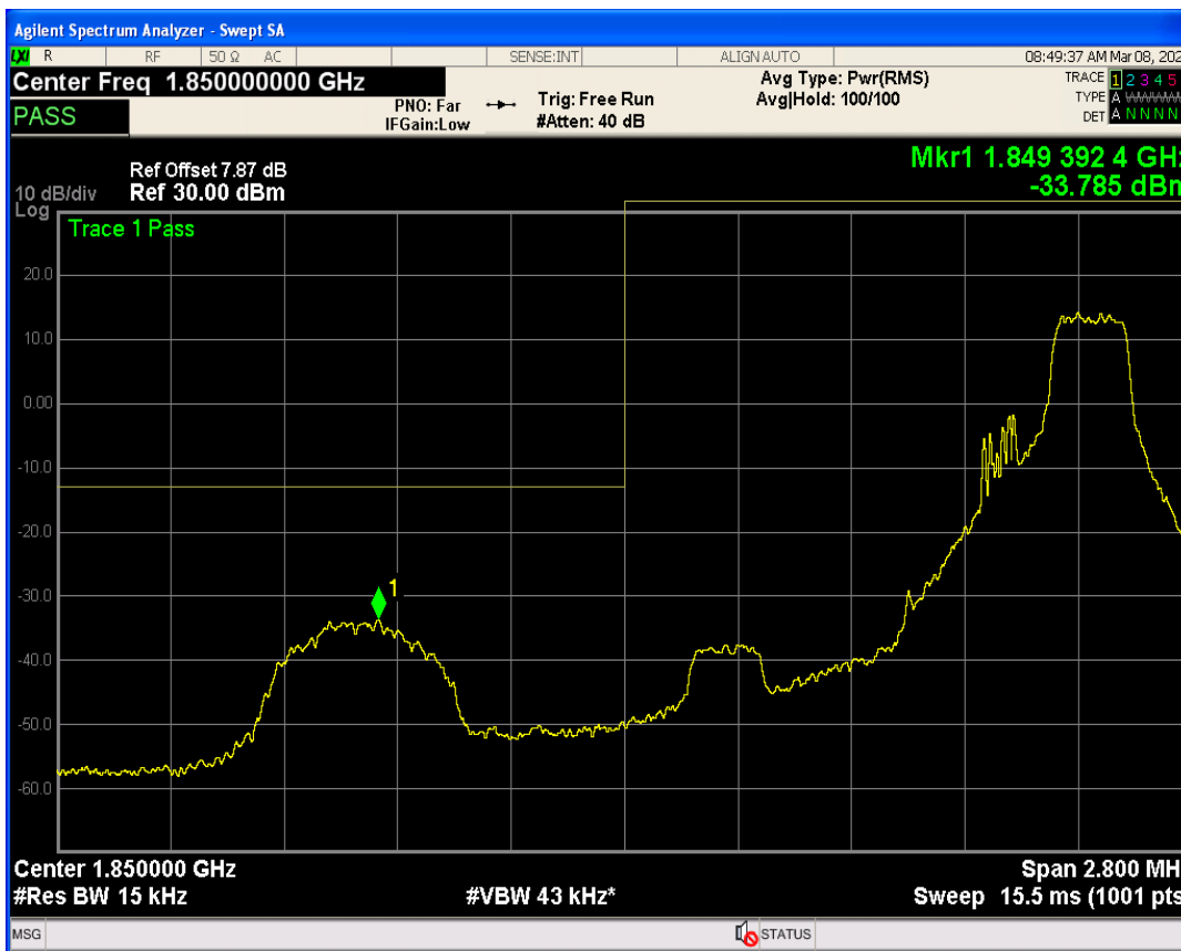
Band2 QPSK BW=1.4MHz Channel=18607 RB Size=1 Position=#0
