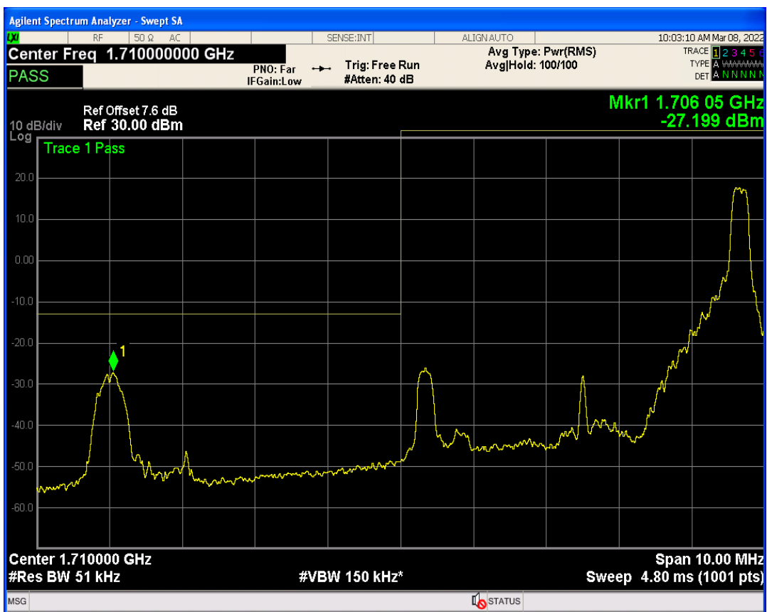
Band4 QPSK BW=5MHz Channel=19975 RB Size=1 Position=#0
