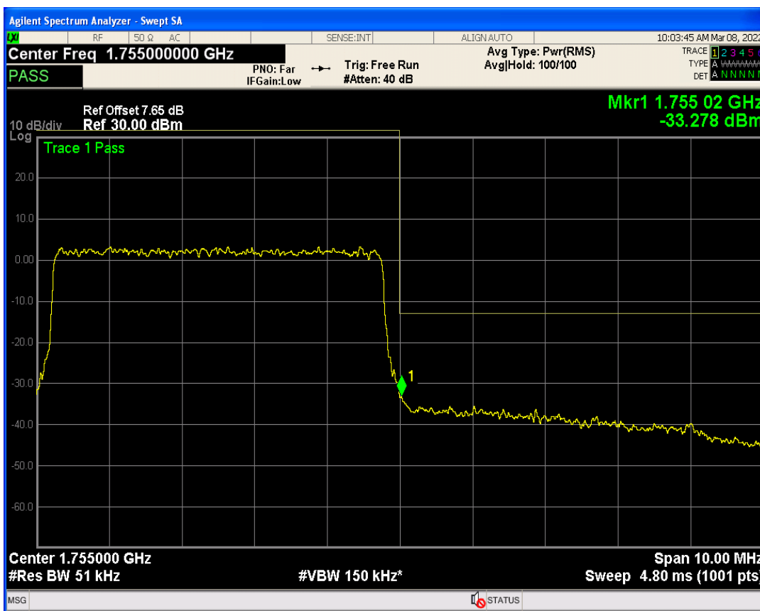
Band4 QPSK BW=10MHz Channel=20000 RB Size=50 Position=#0
