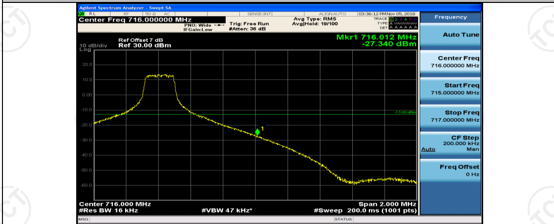
Channel Bandwidth: 10 MHz_HCH_QPSK_25RB#0
