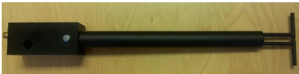
Figure 1 – MVG COMOSAR Validation Dipole
