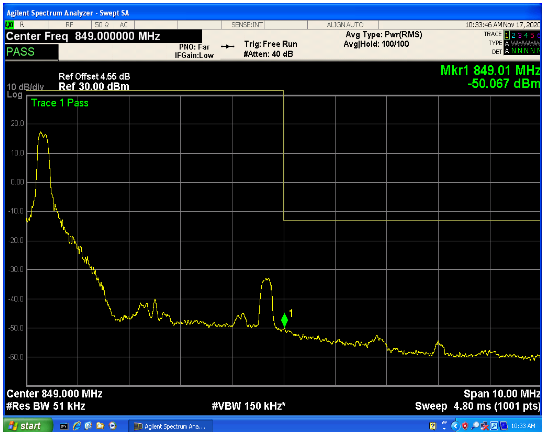
LTE Band5 QPSK BW=5MHz Channel=20625 RB Size=25 Position=#0
