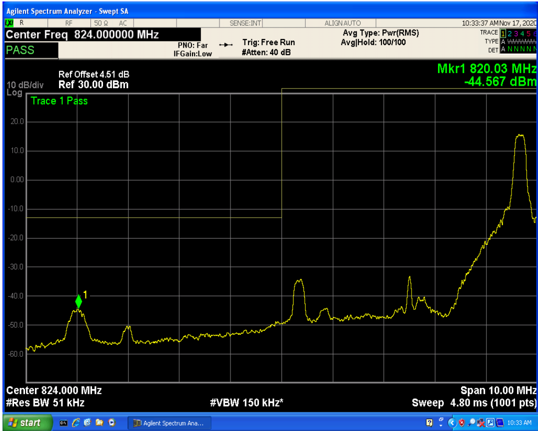
LTE Band5 QAM16 BW=5MHz Channel=20425 RB Size=25 Position=#0
