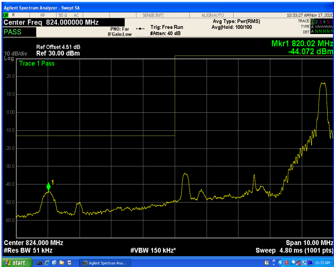
LTE Band5 QPSK BW=5MHz Channel=20425 RB Size=25 Position=#0
