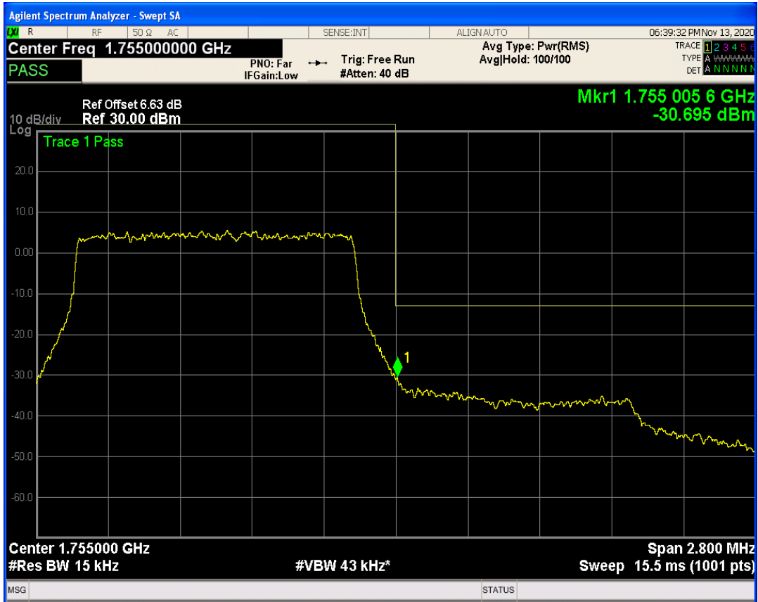
LTE Band4 QAM16 BW=1.4MHz Channel=20393 RB Size=1 Position=#0
