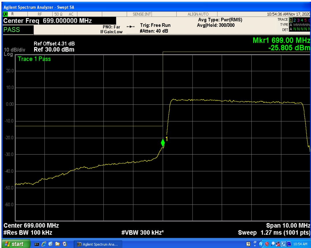
LTE Band12 QPSK BW=5MHz Channel=23155 RB Size=1 Position=#0
