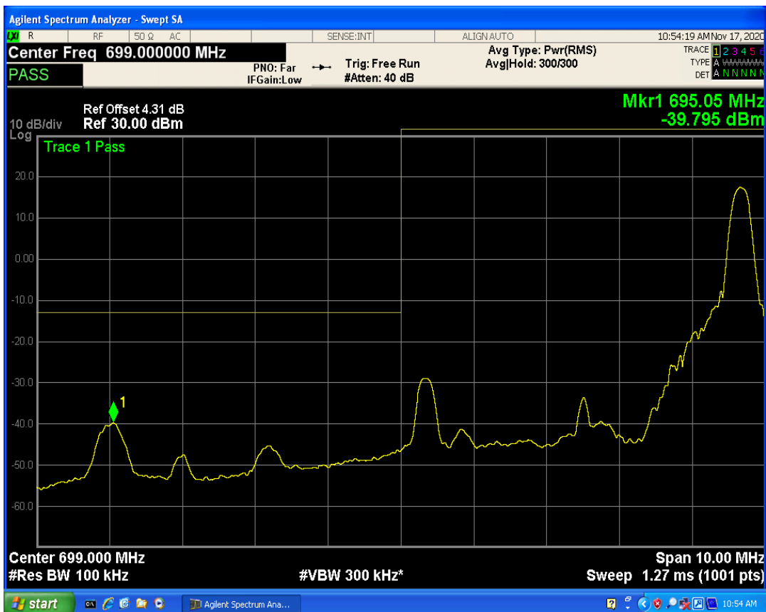
LTE Band12 QPSK BW=5MHz Channel=23035 RB Size=25 Position=#0
