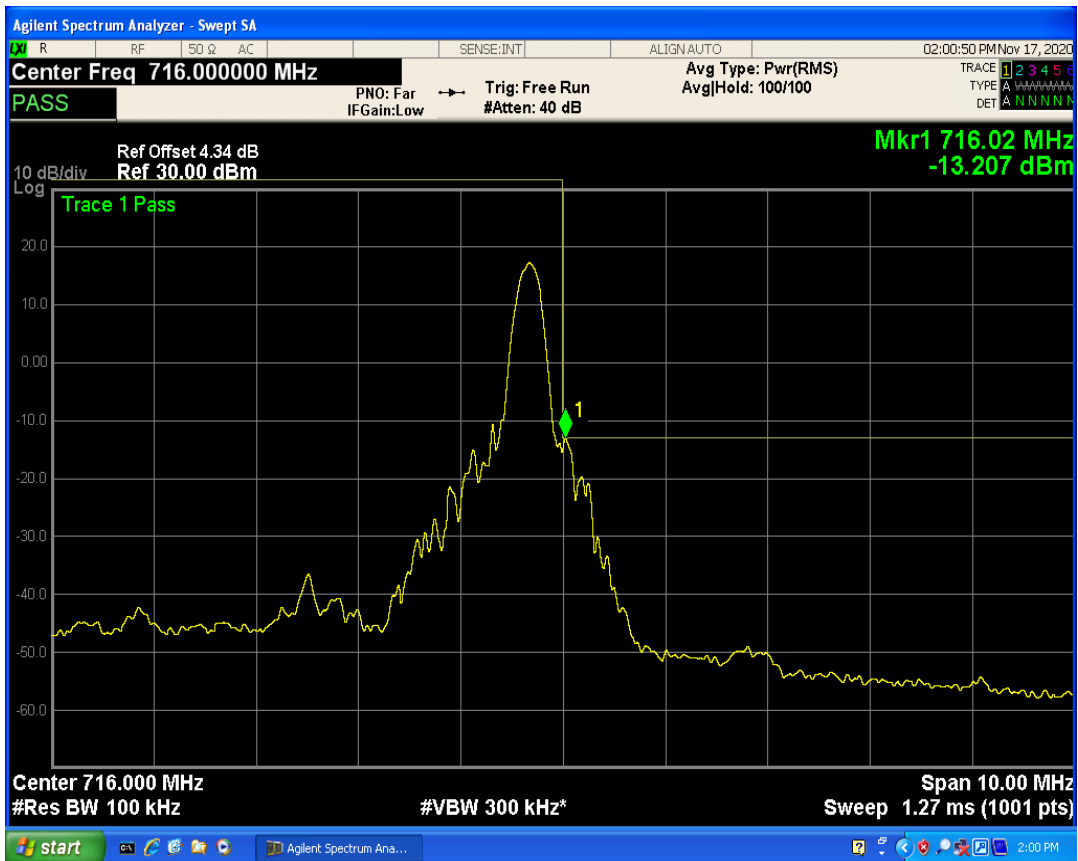
LTE Band17 QAM16 BW=5MHz Channel=23825 RB Size=25 Position=#0
