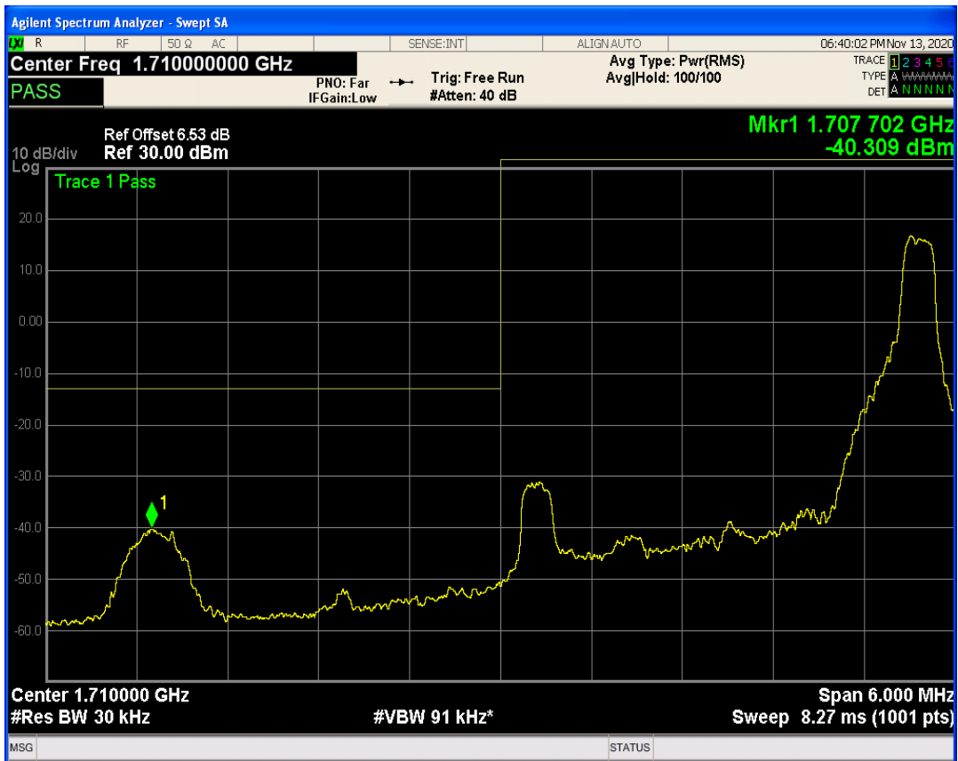
LTE Band4 QAM16 BW=3MHz Channel=19965 RB Size=1 Position=#0
