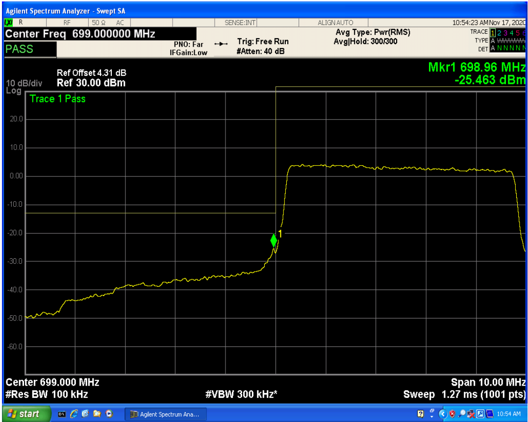
LTE Band12 QAM16 BW=5MHz Channel=23035 RB Size=1 Position=#0
