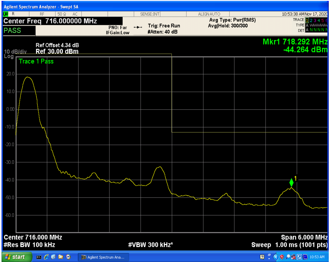
LTE Band12 QPSK BW=3MHz Channel=23165 RB Size=1 Position=#Max
