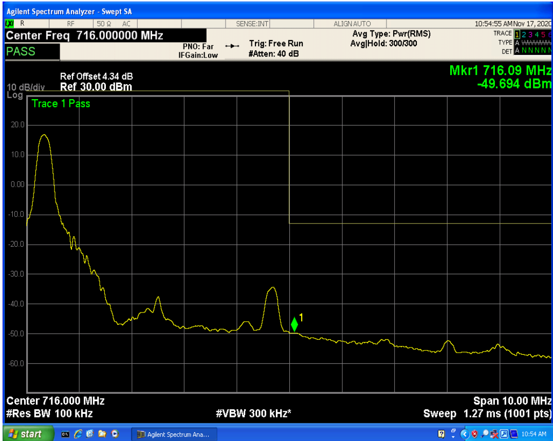
LTE Band12 QPSK BW=5MHz Channel=23155 RB Size=25 Position=#0
