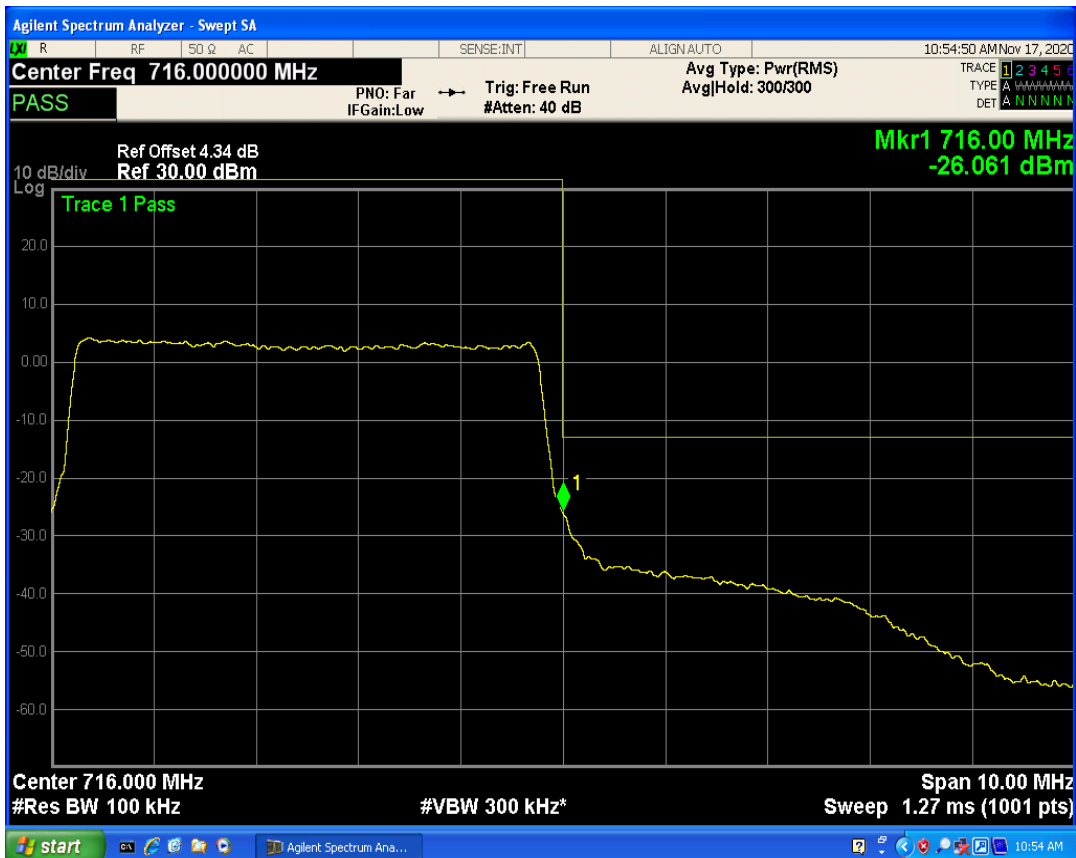
LTE Band12 QAM16 BW=5MHz Channel=23155 RB Size=1 Position=#Max
