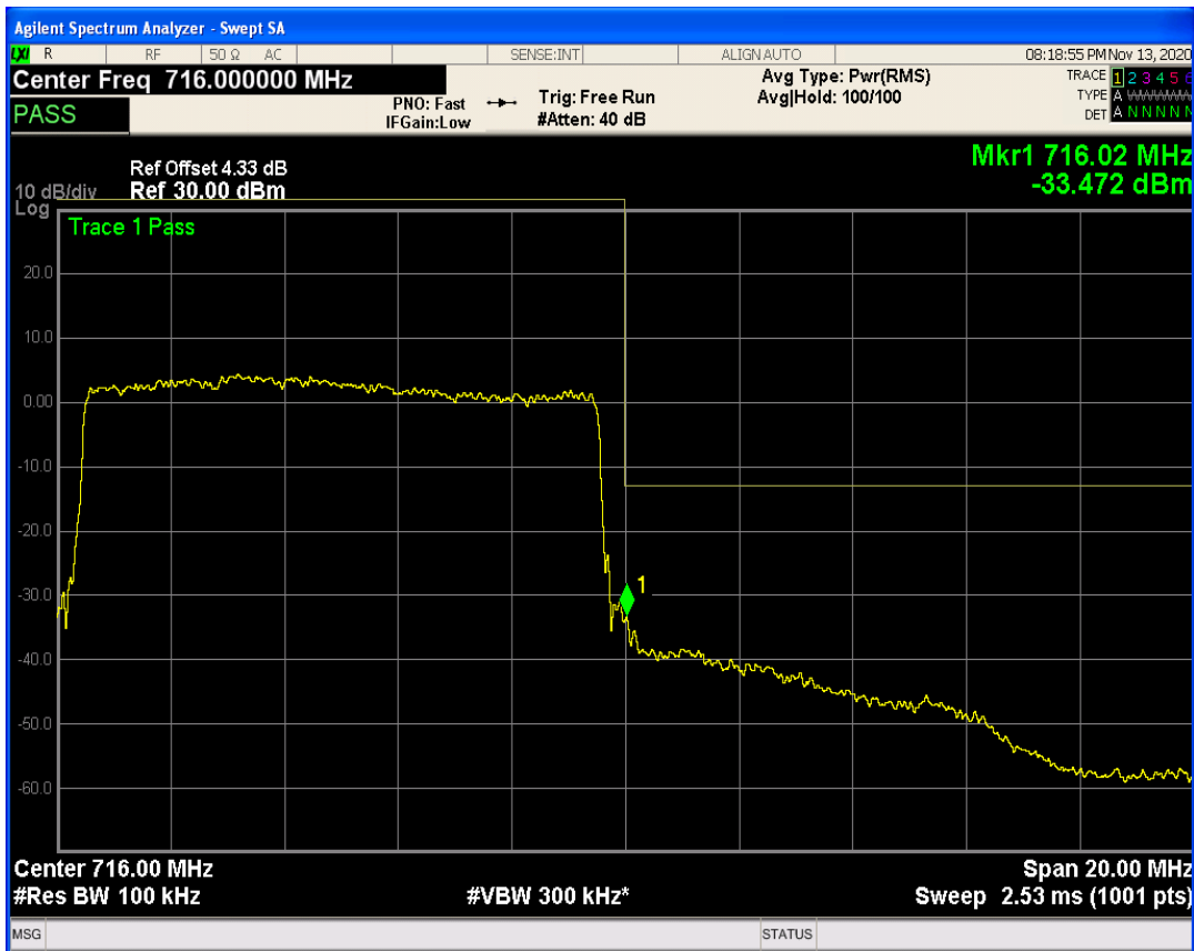
LTE Band17 QPSK BW=5MHz Channel=23825 RB Size=1 Position=#0
