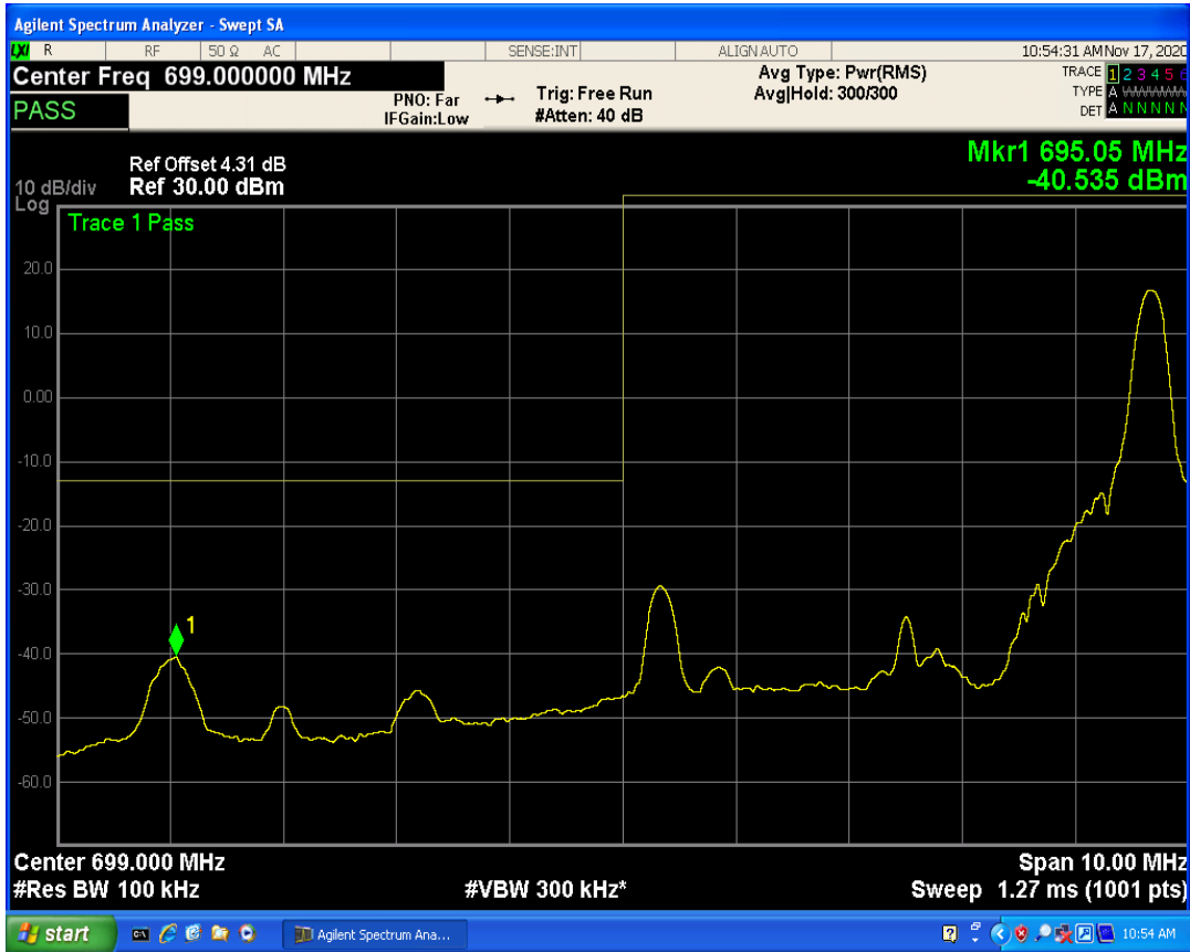
LTE Band12 QAM16 BW=5MHz Channel=23035 RB Size=25 Position=#0
