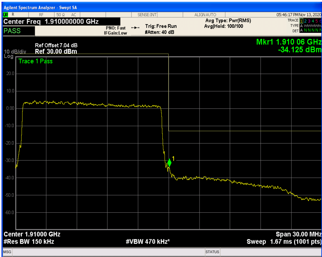
LTE Band2 QAM16 BW=15MHz Channel=19125 RB Size=1 Position=#0
