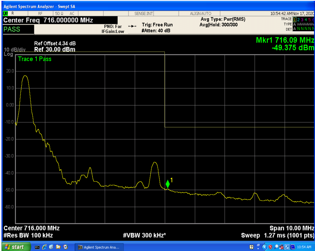
LTE Band12 QPSK BW=5MHz Channel=23155 RB Size=1 Position=#Max
