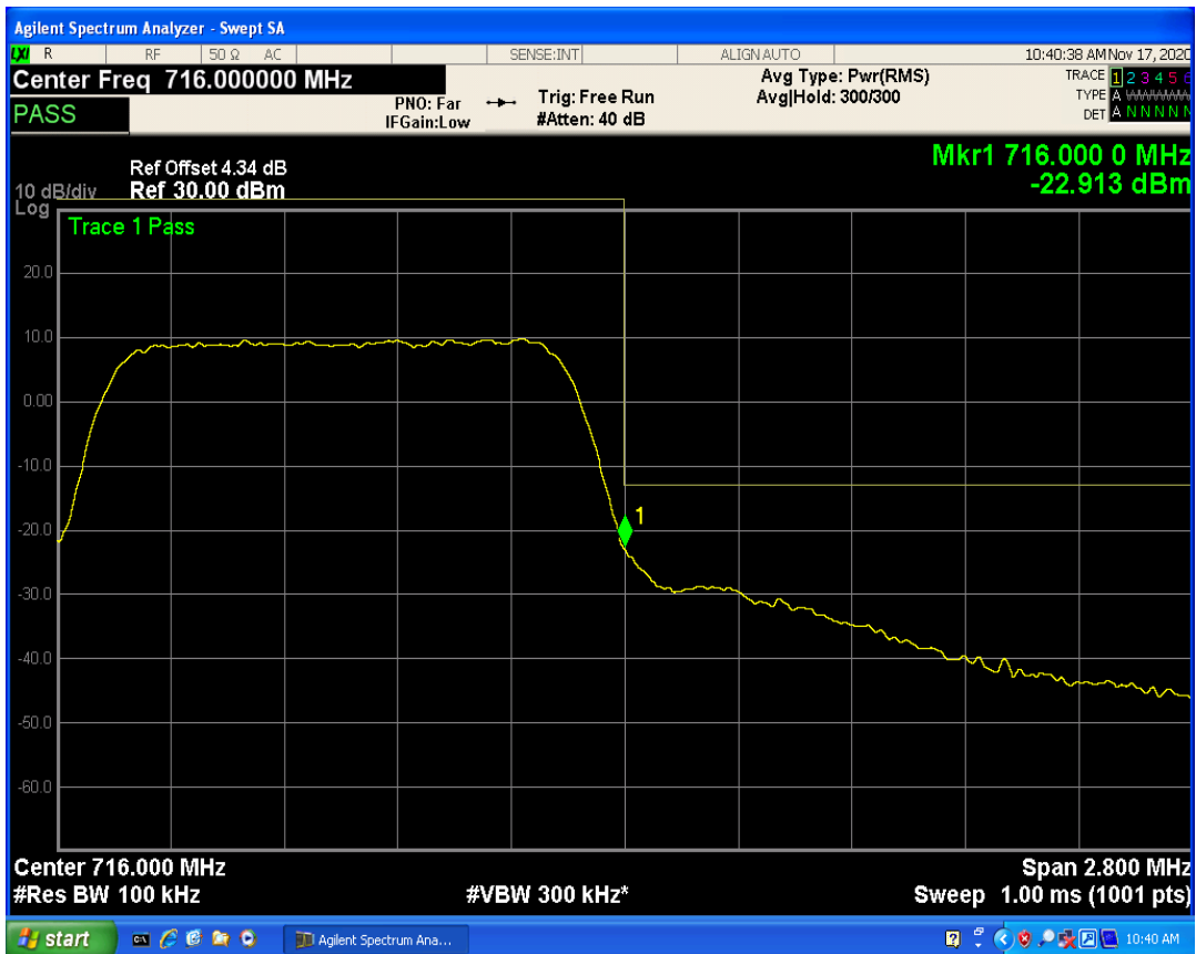
LTE Band12 QPSK BW=10MHz Channel=23060 RB Size=1 Position=#0
