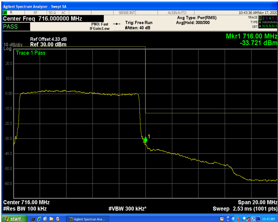
LTE Band12 QAM16 BW=10MHz Channel=23130 RB Size=1 Position=#Max
