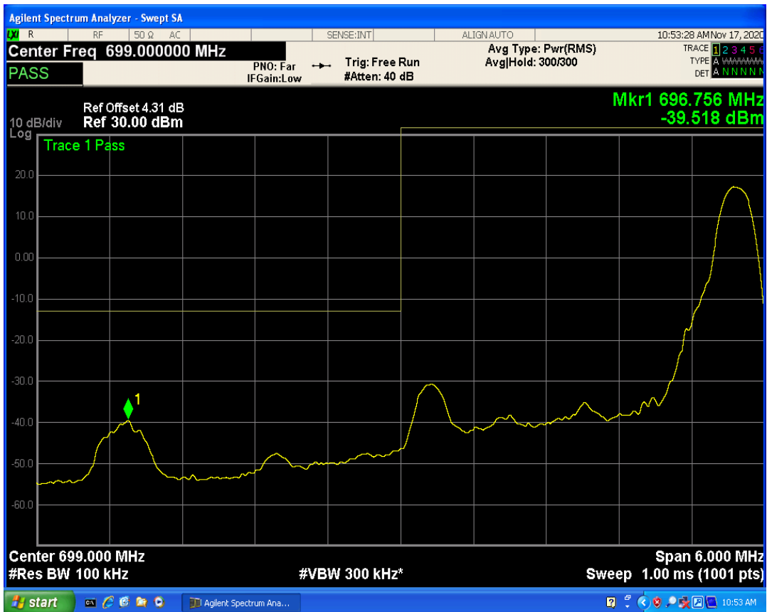
LTE Band12 QPSK BW=3MHz Channel=23165 RB Size=1 Position=#0
