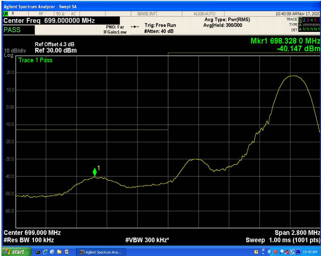
LTE Band12 QAM16 BW=1.4MHz Channel=23017 RB Size=6 Position=#0
