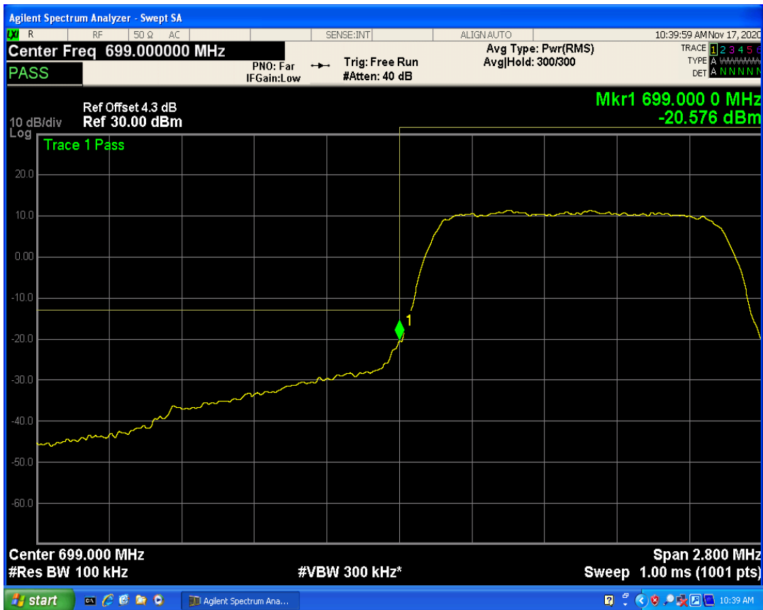
LTE Band12 QAM16 BW=1.4MHz Channel=23017 RB Size=1 Position=#Max
