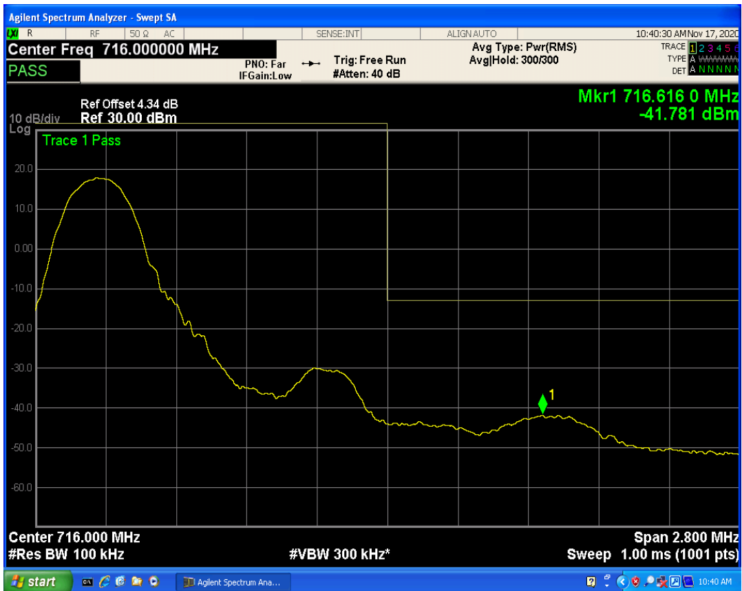
LTE Band12 QAM16 BW=1.4MHz Channel=23173 RB Size=1 Position=#Max
