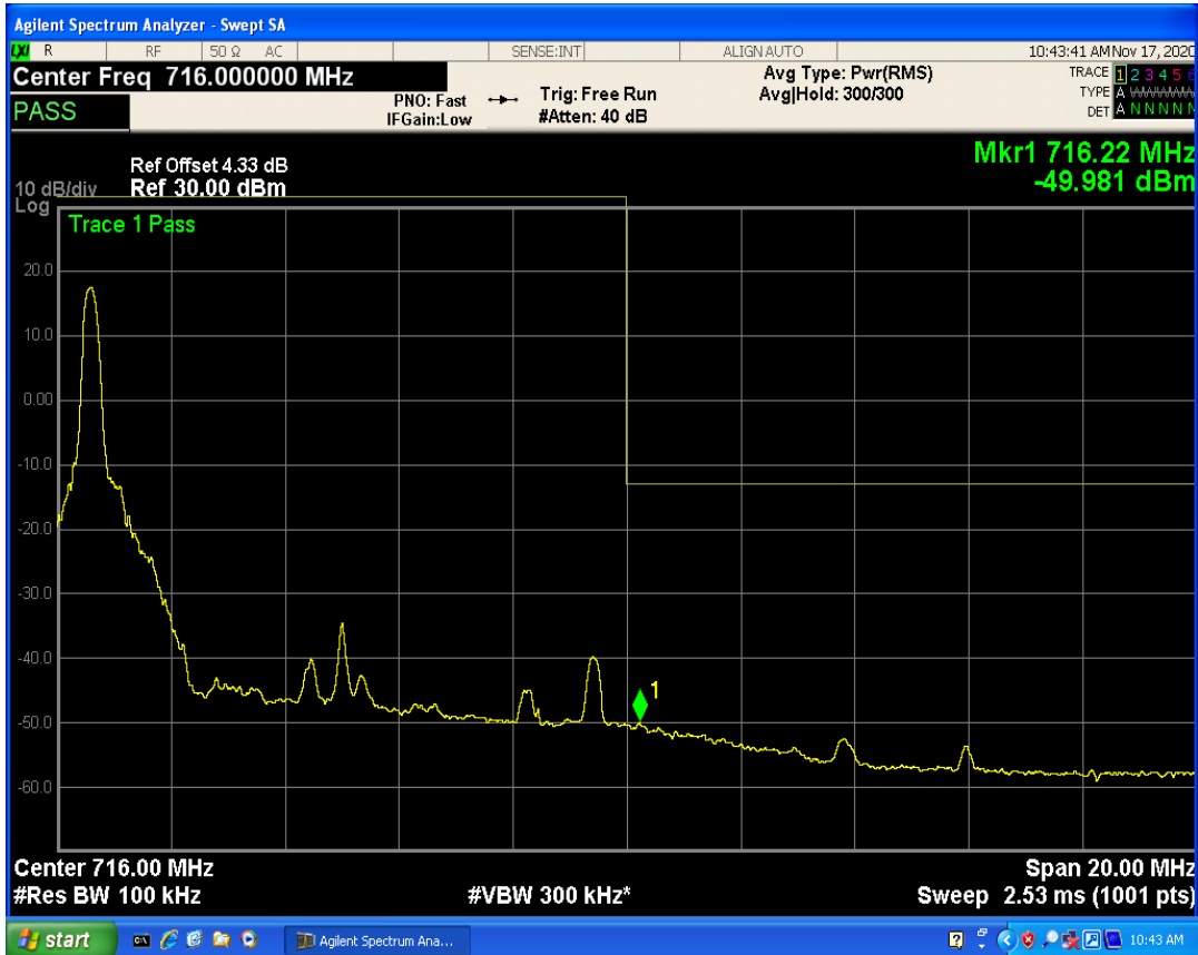
LTE Band12 QPSK BW=10MHz Channel=23130 RB Size=50 Position=#0
