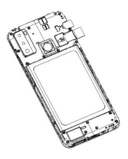
Remove the battery, and install SIM and SD cards, place the cards with chip facing downwards, and then slide it into its slot. Make sure that it is correctly inserted.
