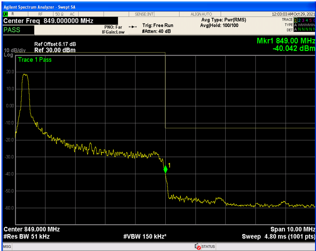
Band5 QPSK BW=5MHz Channel=20625 RB Size=1 Position=#0
