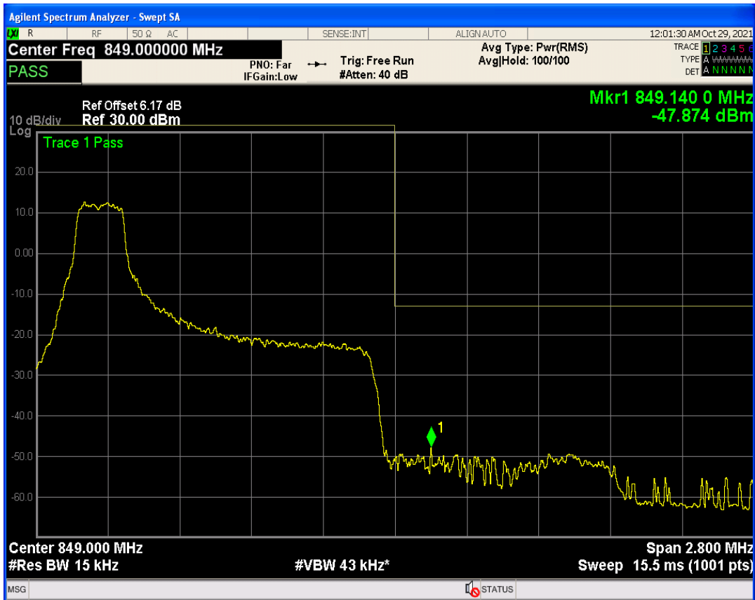
Band5 QAM16 BW=1.4MHz Channel=20643 RB Size=1 Position=#0
