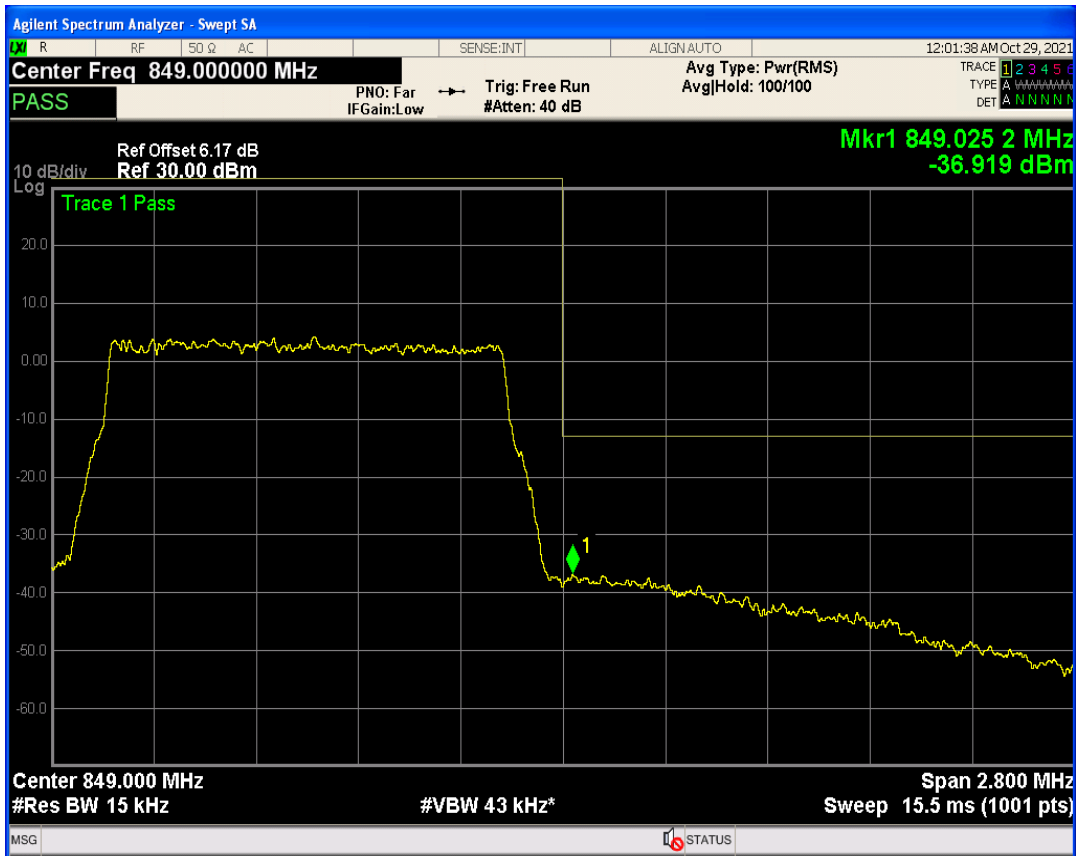
Band5 QPSK BW=3MHz Channel=20415 RB Size=1 Position=#0
