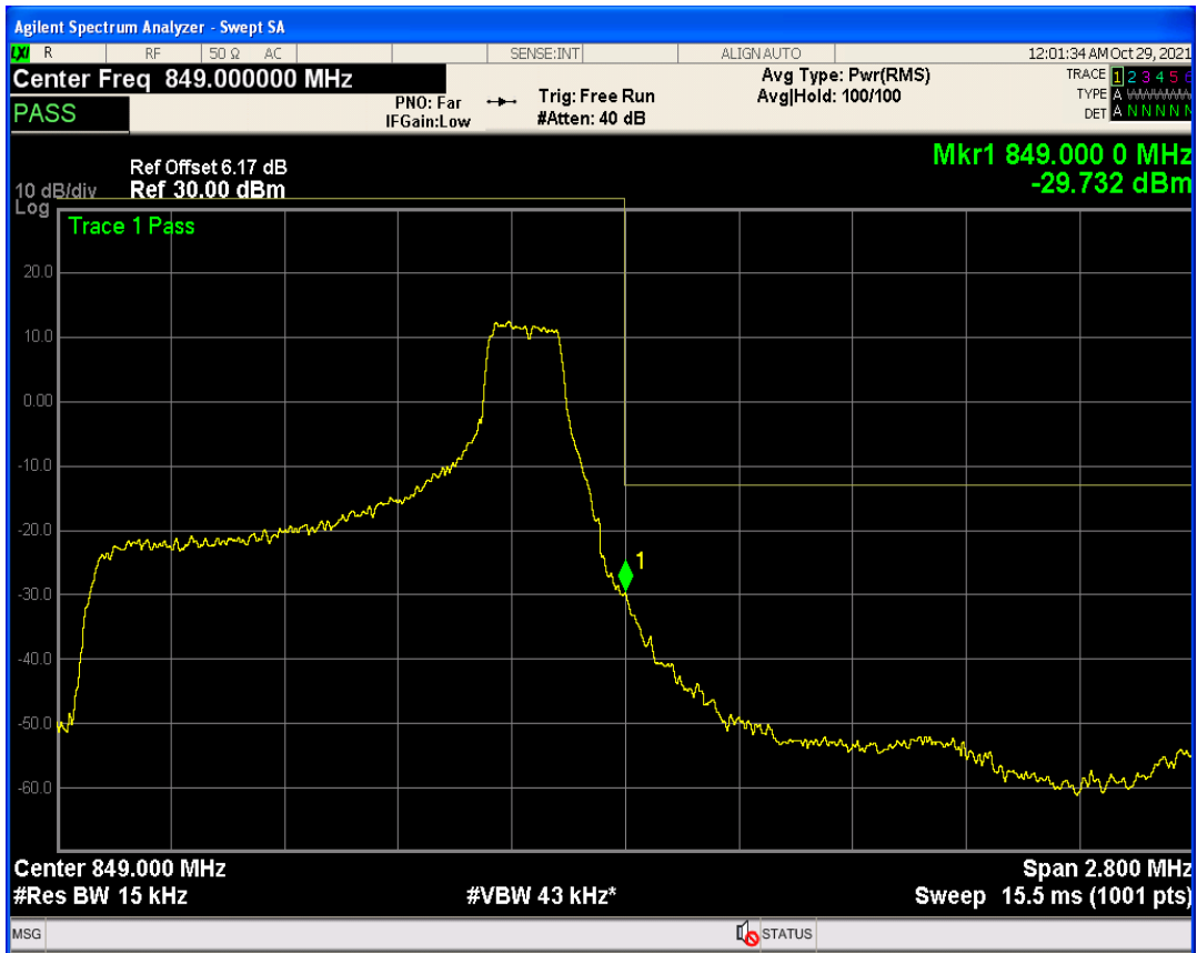
Band5 QAM16 BW=1.4MHz Channel=20643 RB Size=1 Position=#Max
