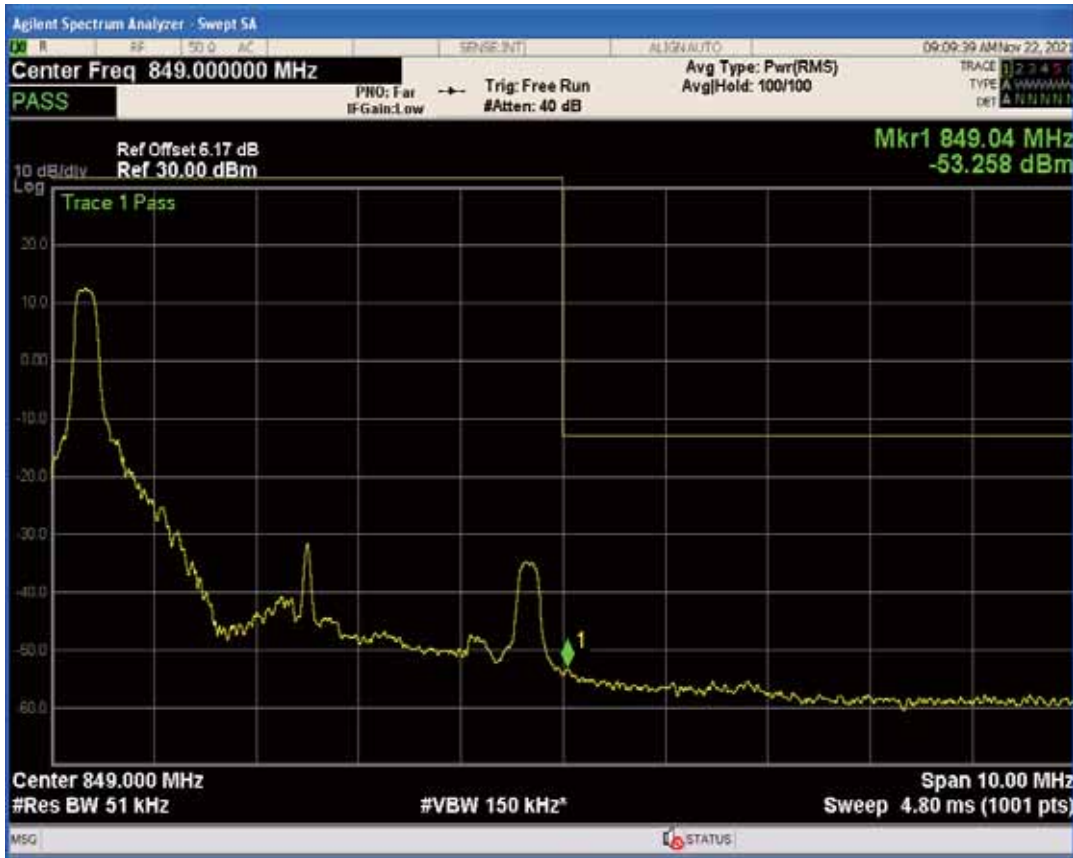
Band7 QPSK BW=5MHz Channel=20775 RB Size=1 Position=#0
