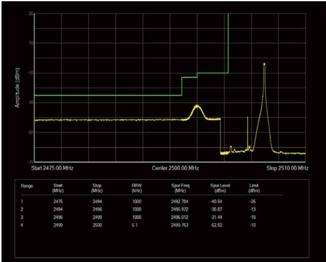
Band7 QPSK BW=5MHz Channel=20775 RB Size=25 Position=#0
