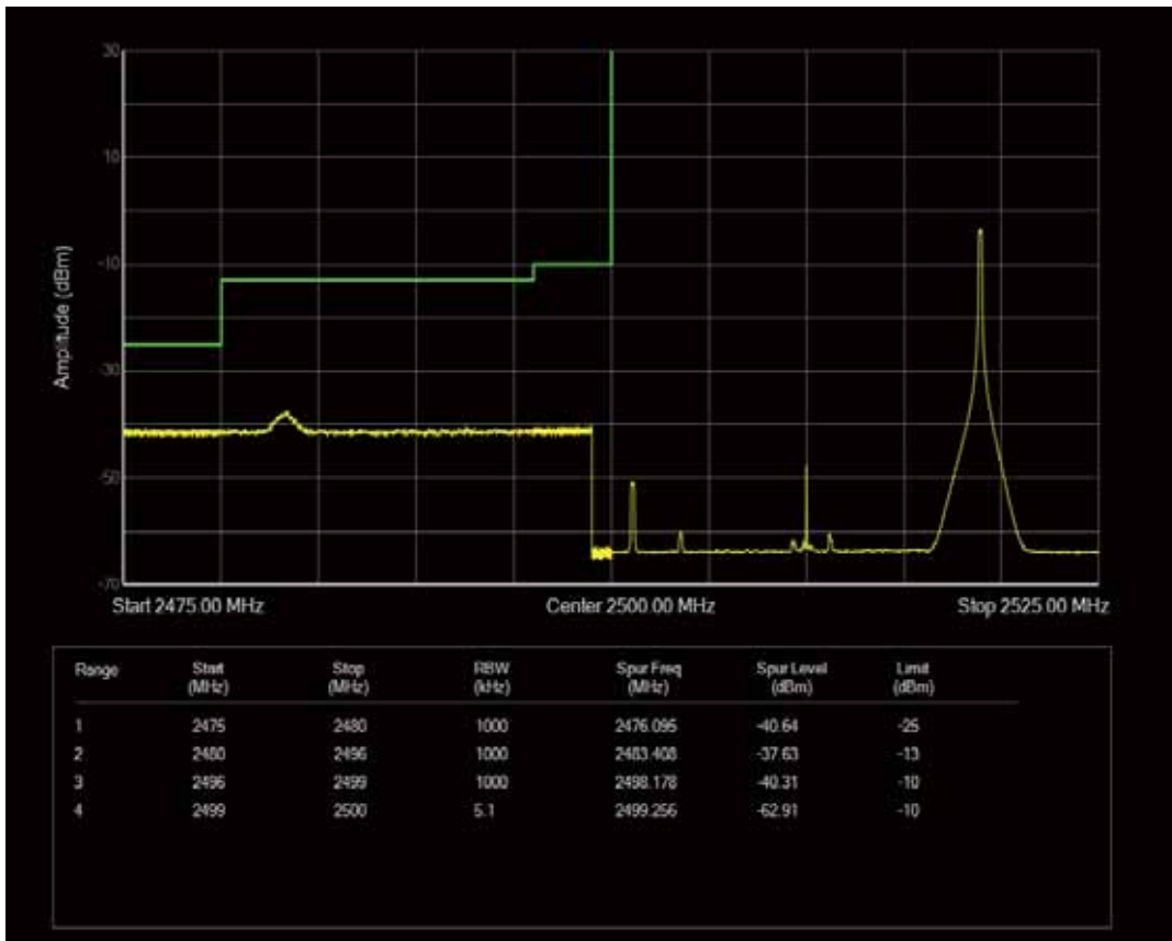
Band7 QPSK BW=20MHz Channel=20850 RB Size=1 Position=#0
