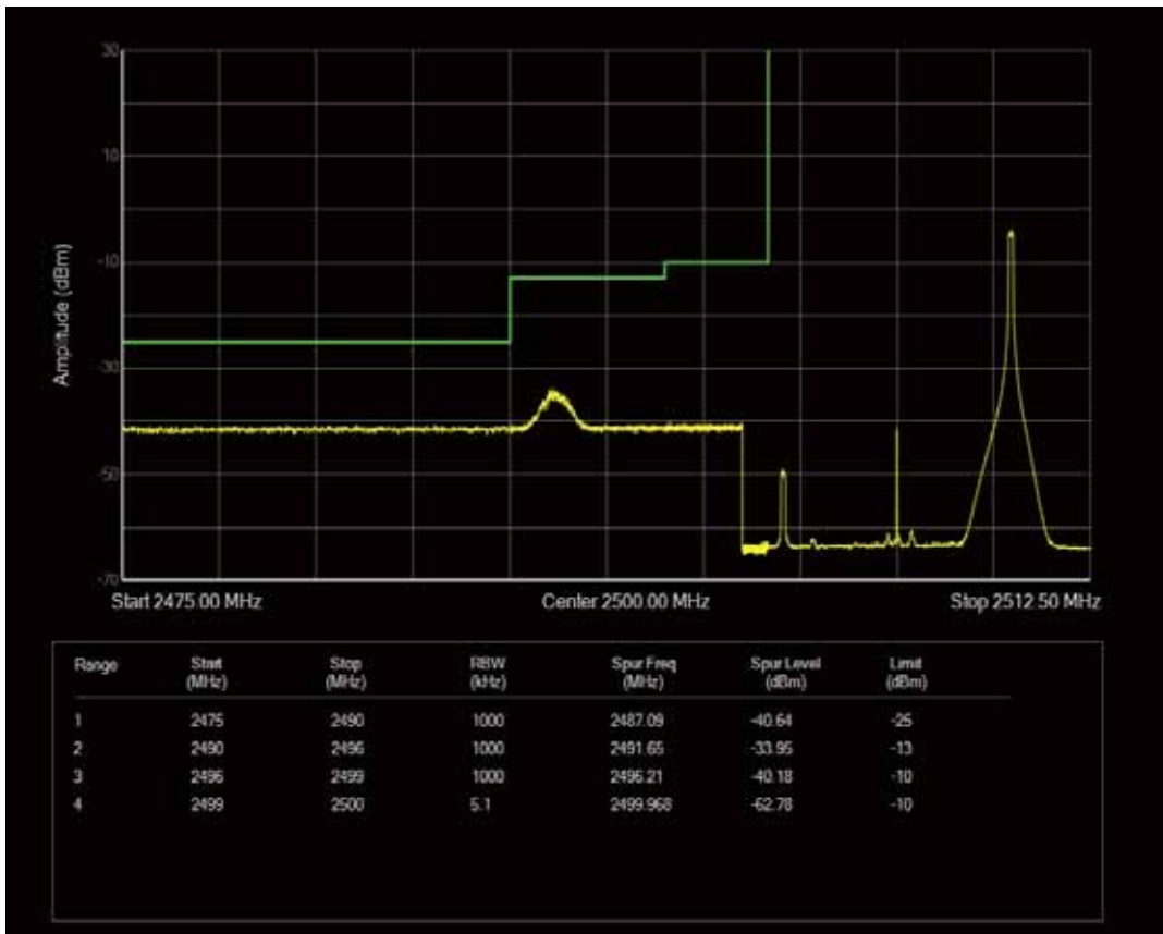
Band7 QAM16 BW=10MHz Channel=20800 RB Size=50 Position=#0
