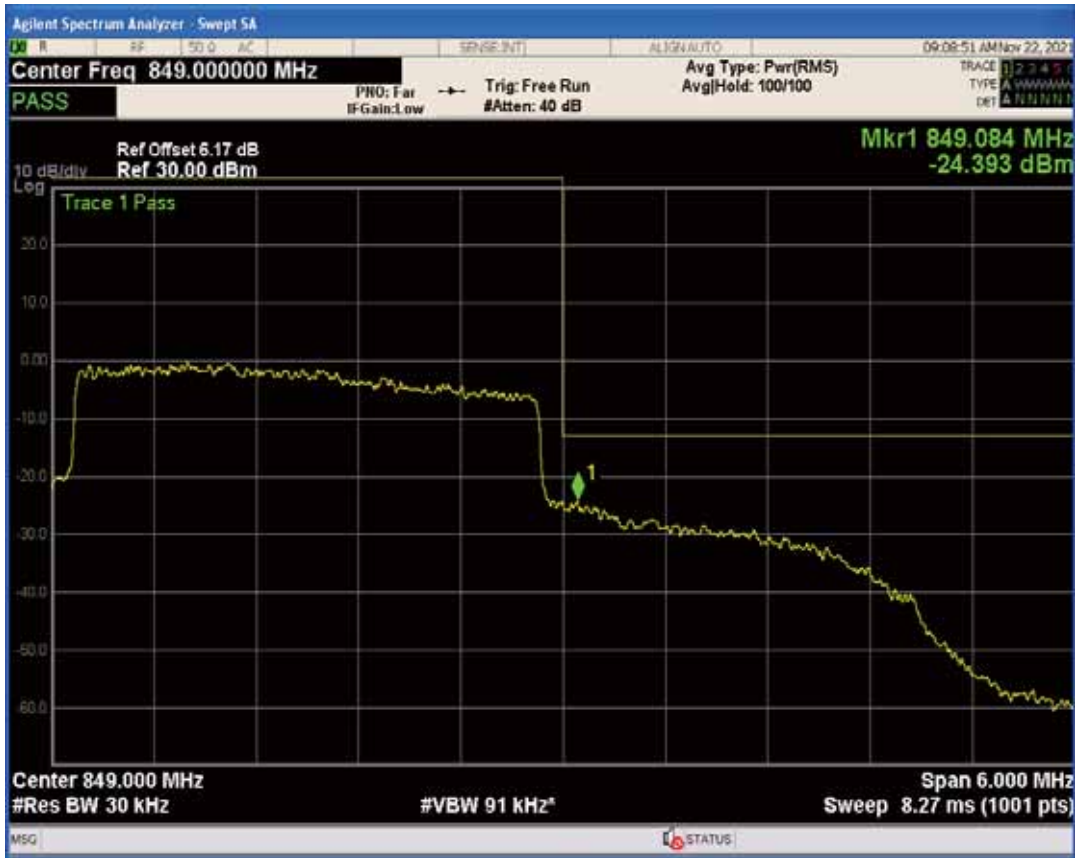
Band5 QPSK BW=5MHz Channel=20425 RB Size=25 Position=#0
