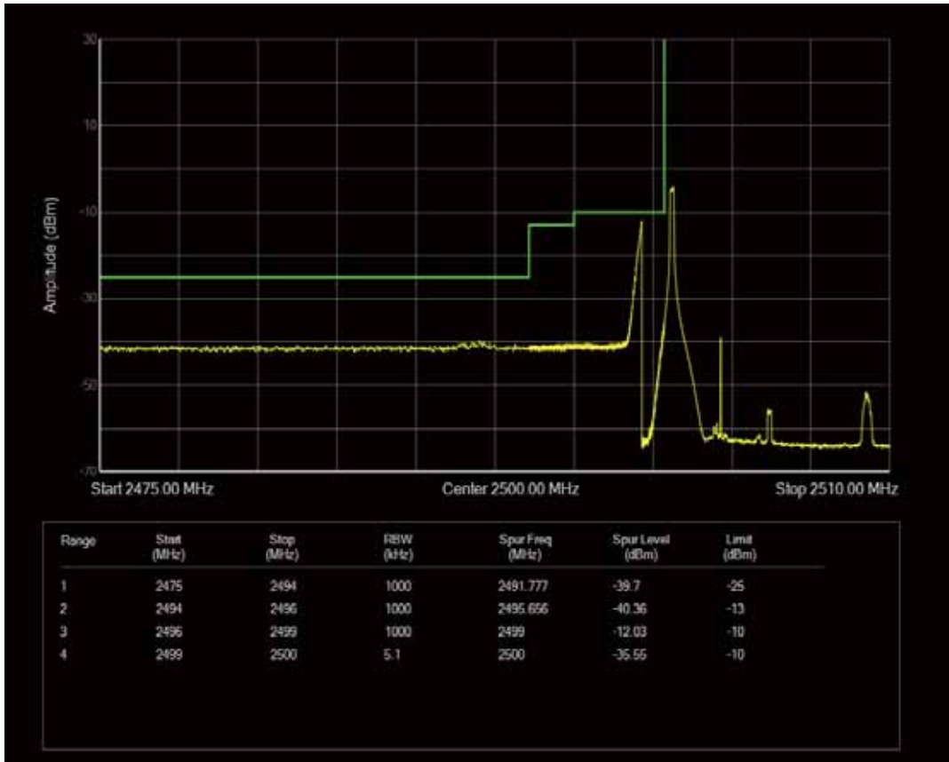
Band7 QAM16 BW=5MHz Channel=20775 RB Size=25 Position=#0
