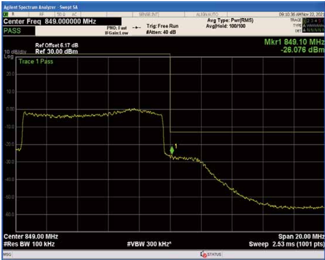
Band5 QPSK BW=10MHz Channel=20600 RB Size=1 Position=#Max
