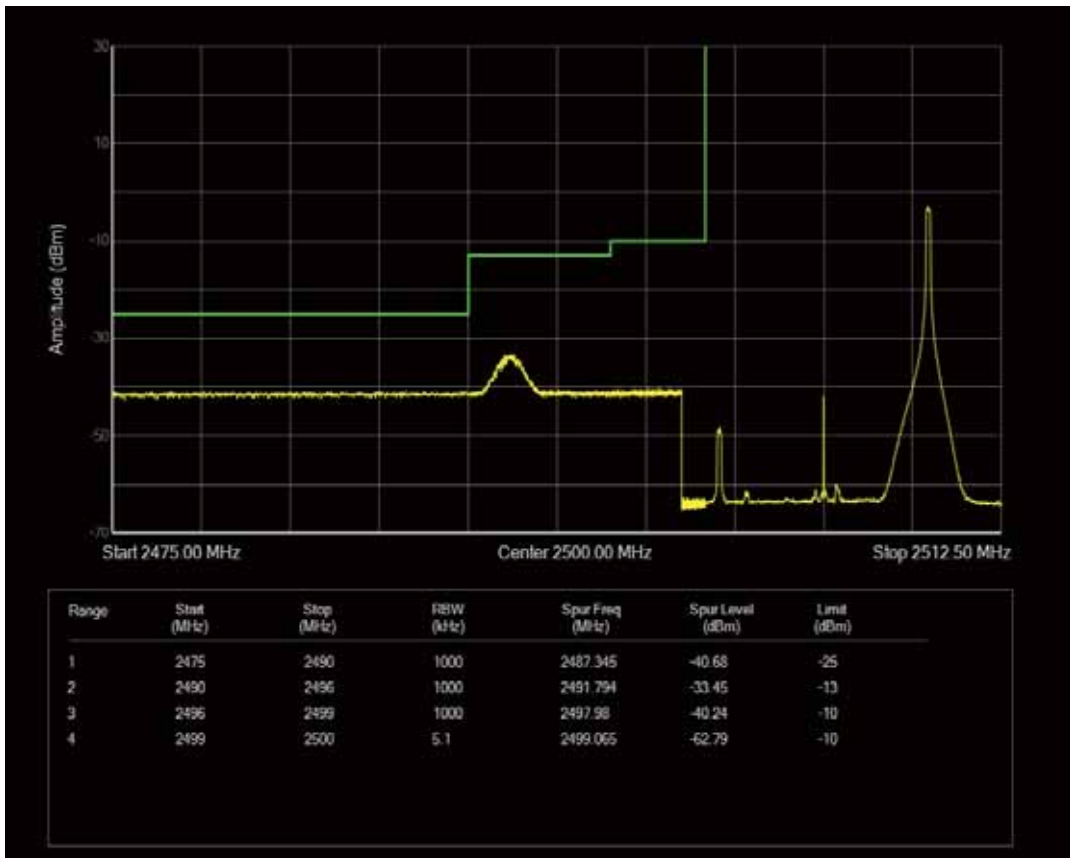
Band7 QPSK BW=10MHz Channel=20800 RB Size=1 Position=#0
