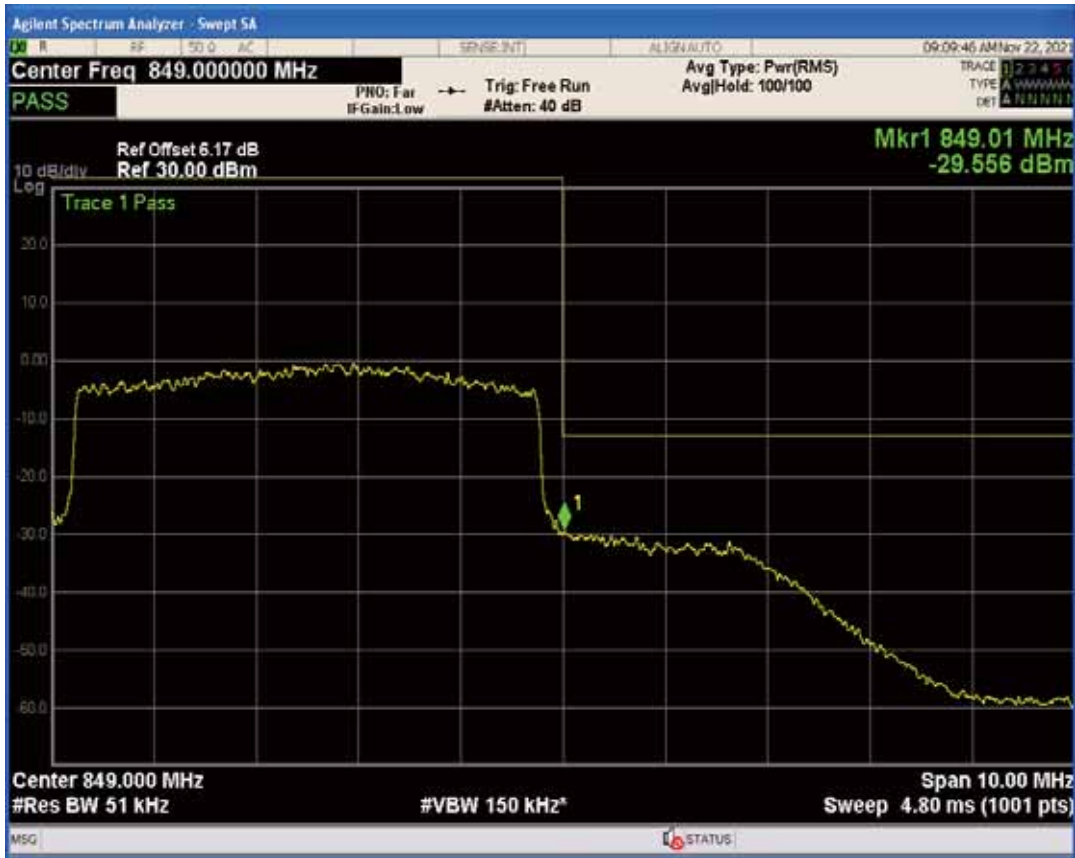
Band5 QPSK BW=5MHz Channel=20625 RB Size=1 Position=#Max
