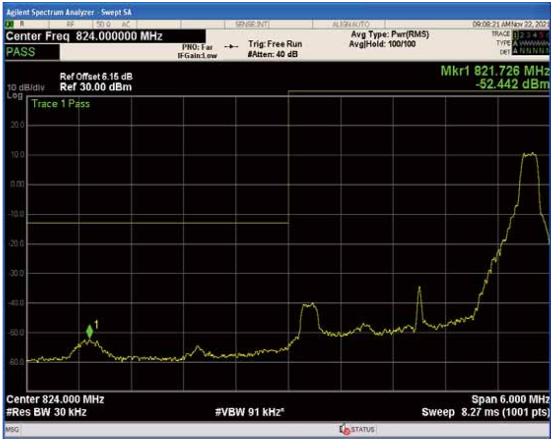
Band5 QPSK BW=10MHz Channel=20450 RB Size=50 Position=#0
