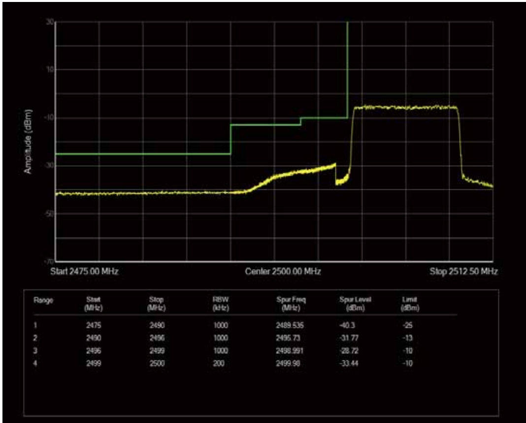
Band7 QAM16 BW=10MHz Channel=20800 RB Size=1 Position=#Max
