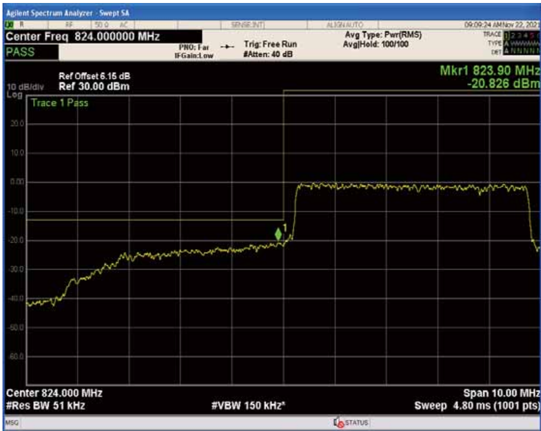
Band5 QPSK BW=5MHz Channel=20425 RB Size=1 Position=#Max
