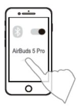
Remark: The device is first paired in the above method; Later, the earbuds can be automatically turned on and connected without the need for pairing.
