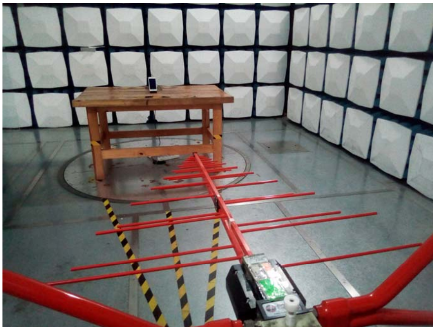
Radiated Emission View (30 MHz ~1 GHz) for Power Transmission
