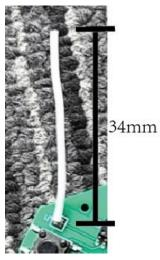
A whip antenna, measuring 34mm in length, is soldered onto the PCB (Printed Circuit Board).
