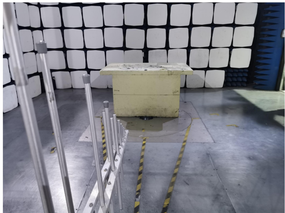
Radiation Emission Test Setup (30MHz to 1GHz)
