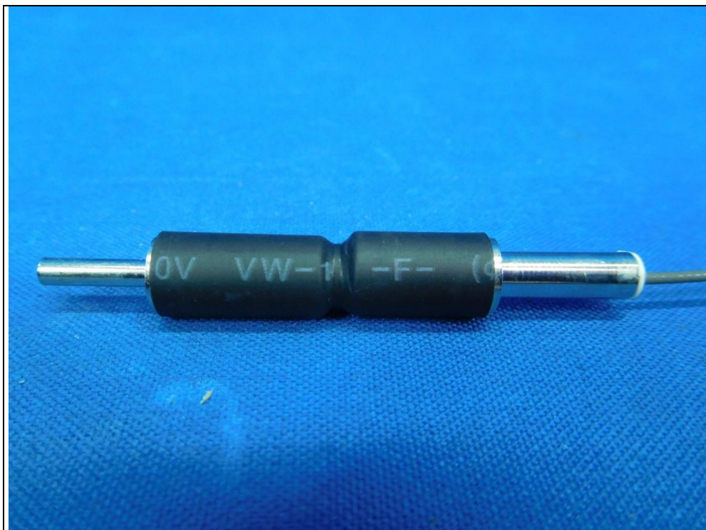
WLAN antenna No. 1
