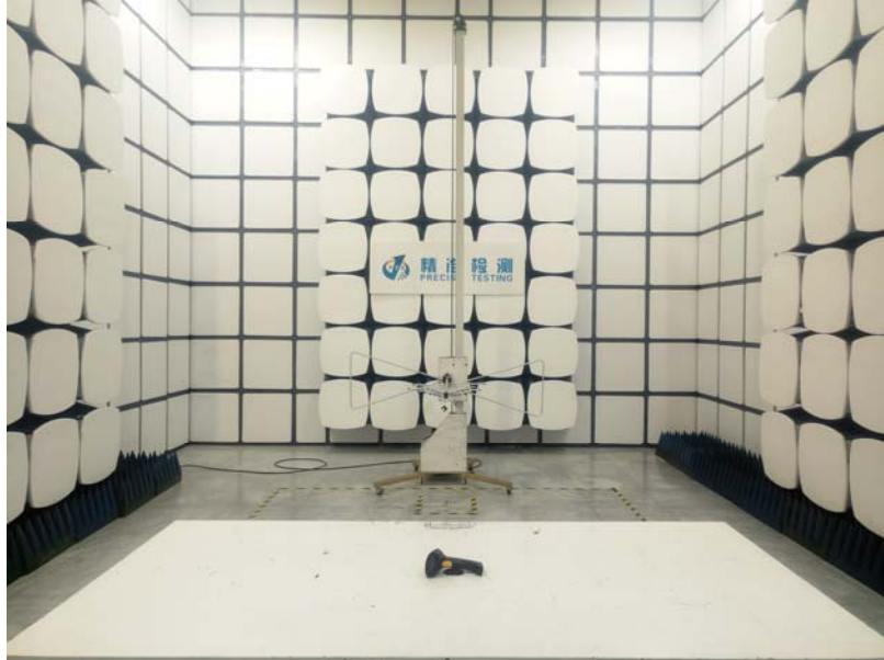
Radiated Spurious Emissions From 30MHz-1000MHz
