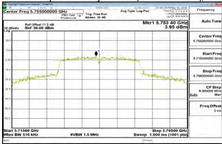
802.11n HT40, 5725~5850 MHz Peak Power Spectral Density Data Plot (CH Low 5755 MHz)
