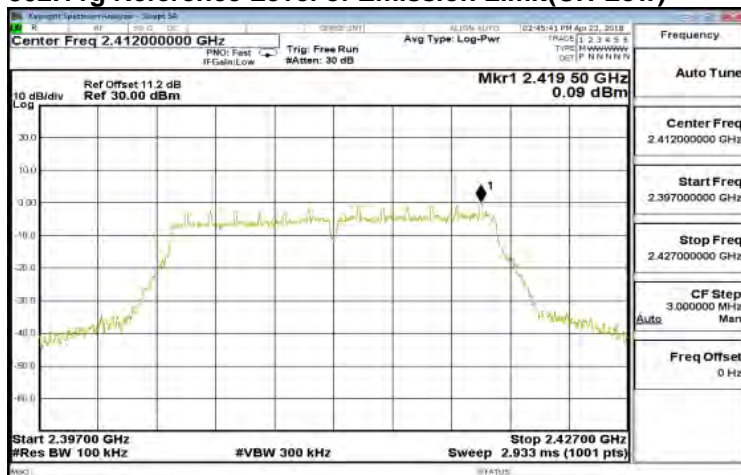
802.11g Reference Level of Emission Limit (CH-Low)
