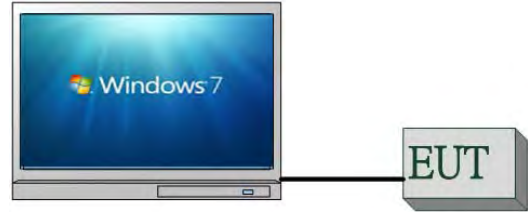
Fig. 2-2 Radiated Emission Configuration
