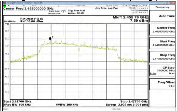
802.11n_HT20 Reference Level of Emission Limit (CH-Low)
