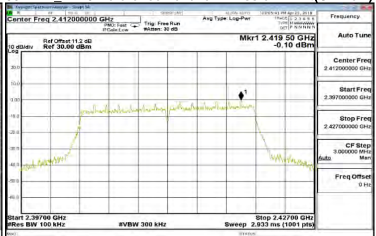
802.11n_HT20 Reference Level of Emission Limit (CH-High)
