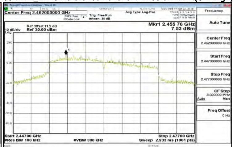
802.11n_HT20 Reference Level of Emission Limit (CH-High)
