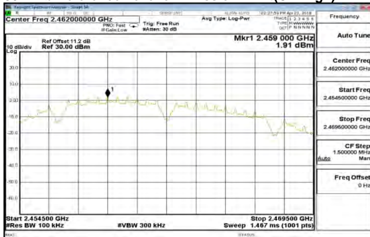
802.11g Reference Level of Emission Limit (CH-Low)
