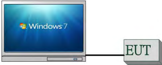
Fig. 2-1 Conducted Emission Configuration
