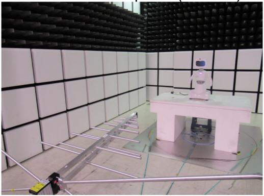
Radiated Emission Set up Photos (Above 1GHz)
