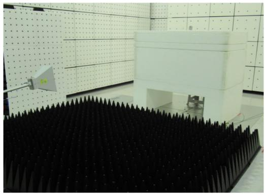
Radiated Emission Set up Photo (Front View)
