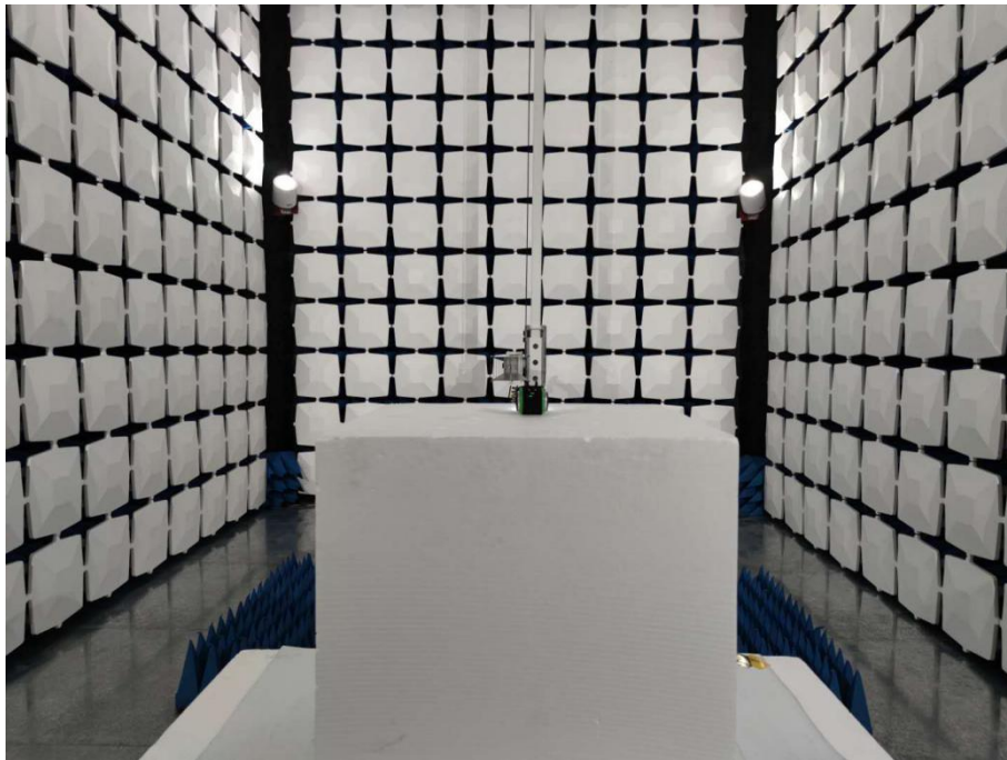
Below 1GHz for radiated emission test setup
