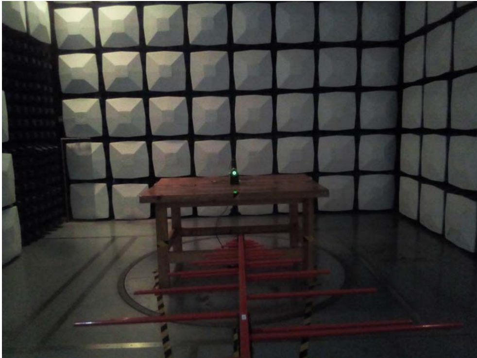
Radiated Emission View (Below 1GHz)
